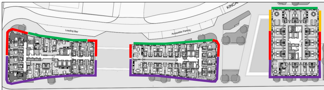
Plan Showing Preliminary Façade Performance Zones (L01-05)
