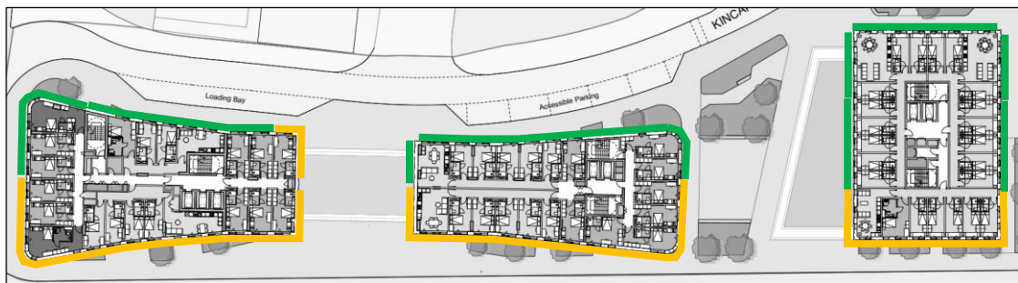
Plan Showing Preliminary Façade Performance Zones (L09-11)
