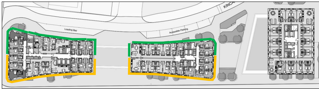
Plan Showing Preliminary Façade Performance Zones (L12-13)
