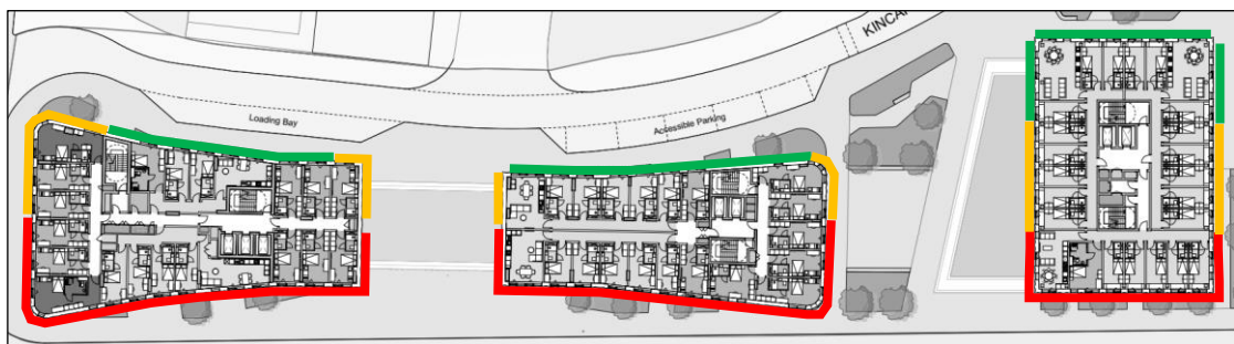
Plan Showing Preliminary Façade Performance Zones (L06-09)
