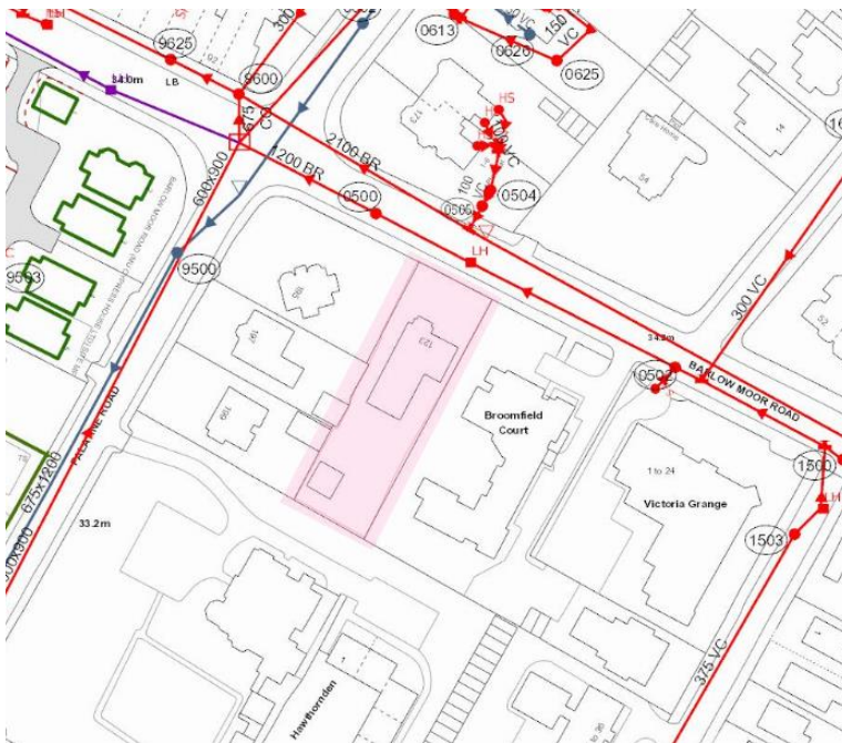
Figure 1 United Utilities Sewer Records
