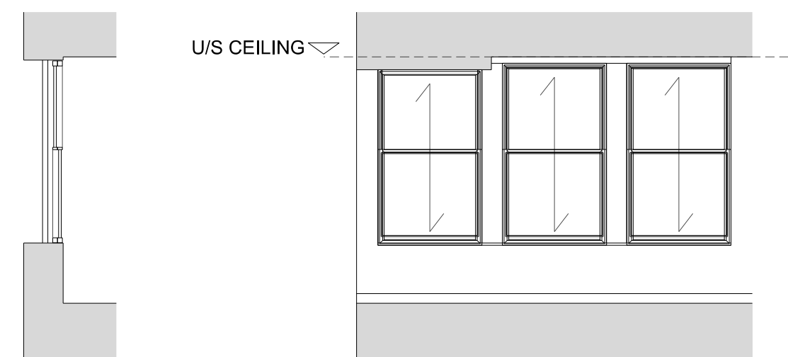
PROPOSED SECTION TYPE K SECONDARY GLAZING 3 NO. VERTICAL SLIDER
