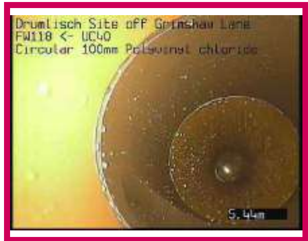
2, 00:00:43, 5.44 m Finish node, other special chamber, reference: UC40, UC40
