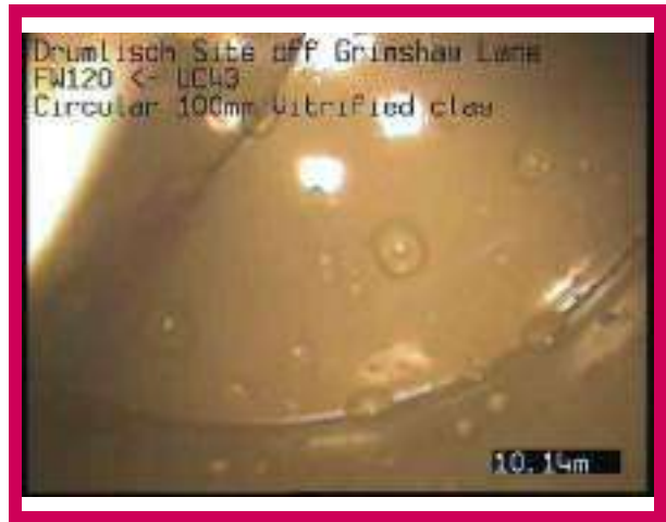
2, 00:00:37, 10.14 m Finish node, other special chamber, reference: UC43, UC43
