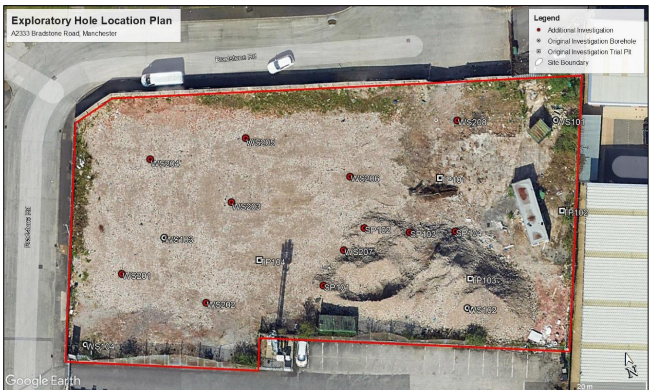
Figure 8 Exploratory Hole Location Plan
