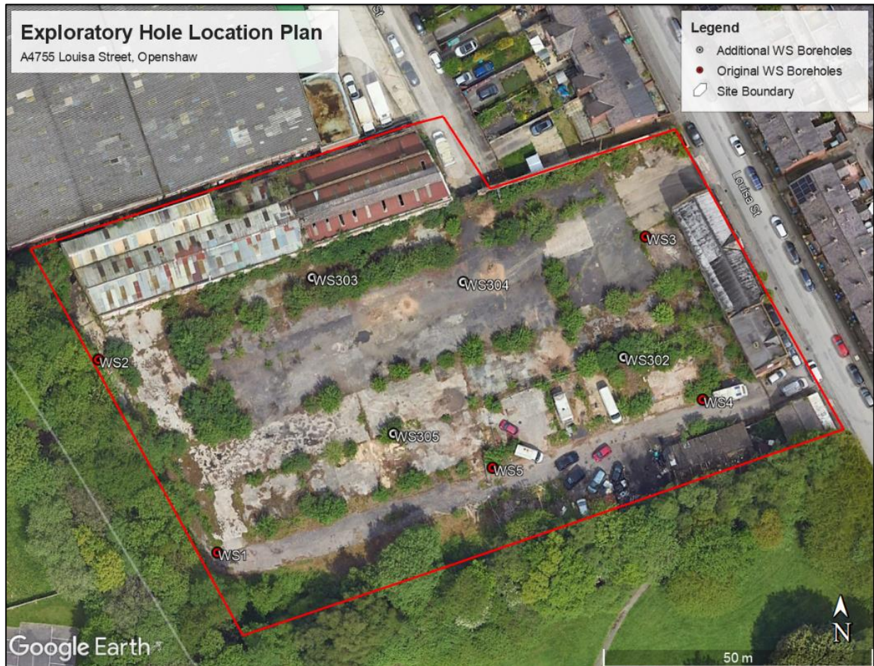
Figure 4 Location of Boreholes WS302 to WS305
