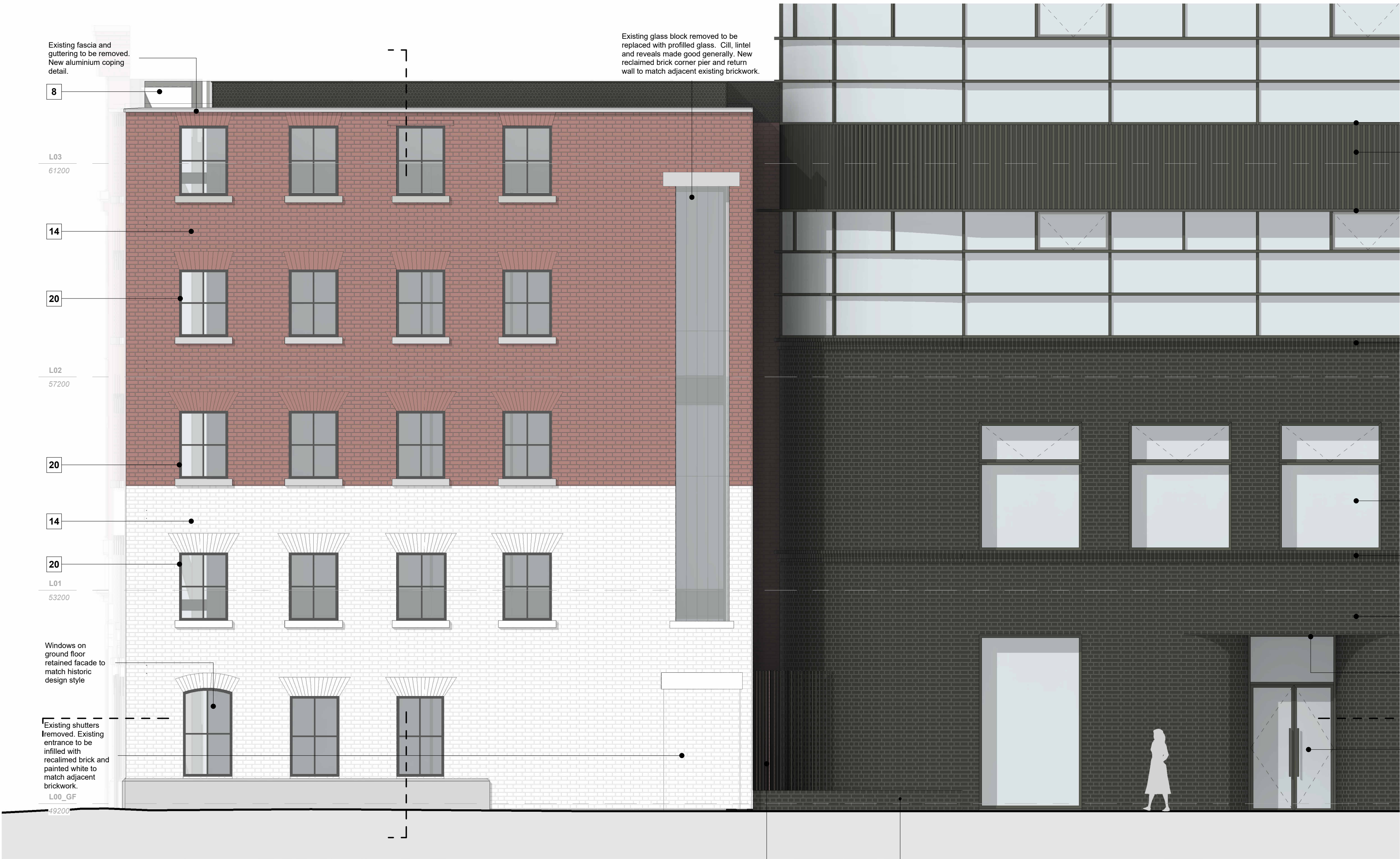
Typical Bay Study 04 - Elevation 1:50
