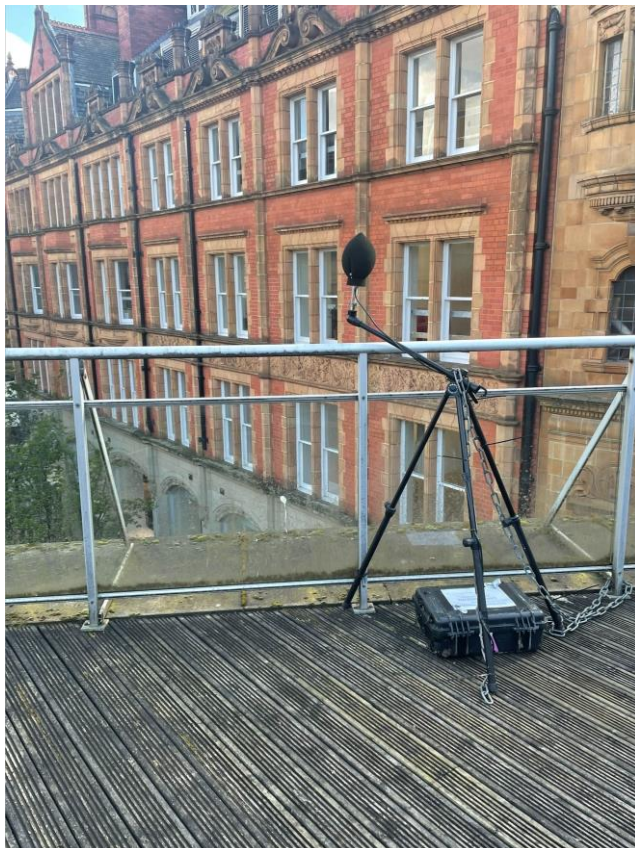
Figure 2 Photograph of unattended measurement position on existing roof terrace
