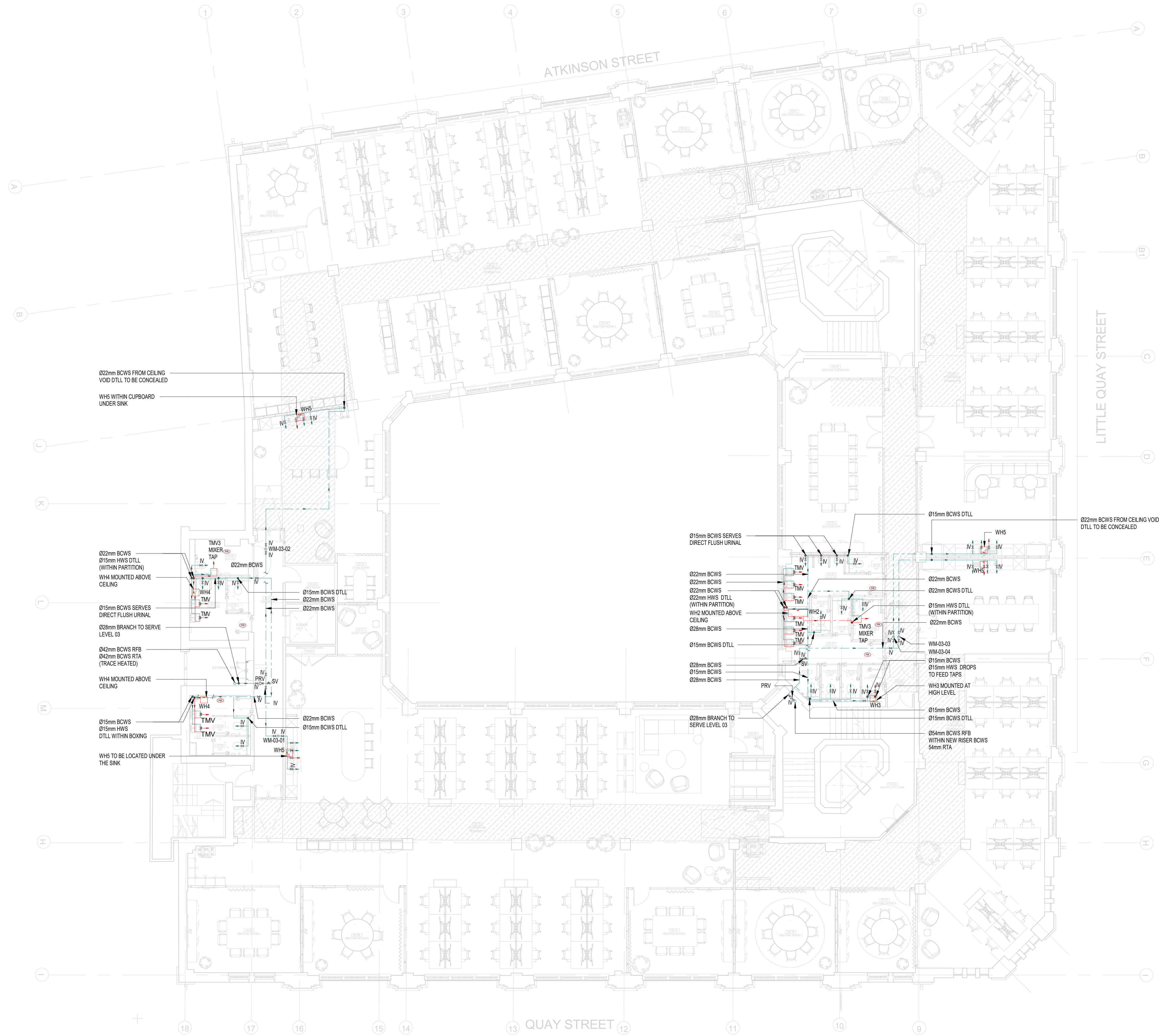
1 MECHANICAL SERVICES DOMESTIC WATER LAYOUT LEVEL 03 1 : 100
