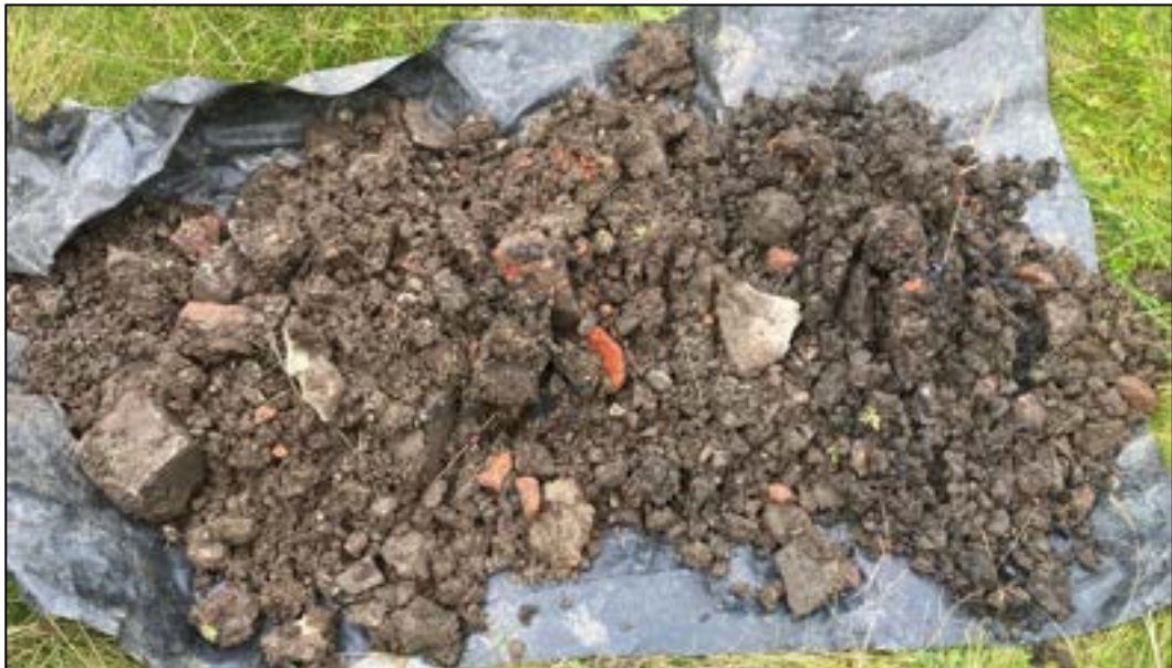
Figure 4-9: Photographic record of the soil profile at HP17, comprising gravelly, fine grained soils
