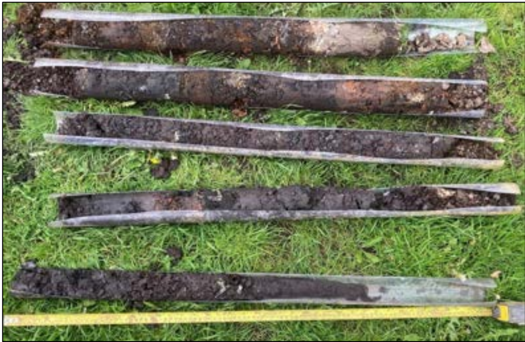
Figure 4-4: Photographic record of soil profile at WS07
