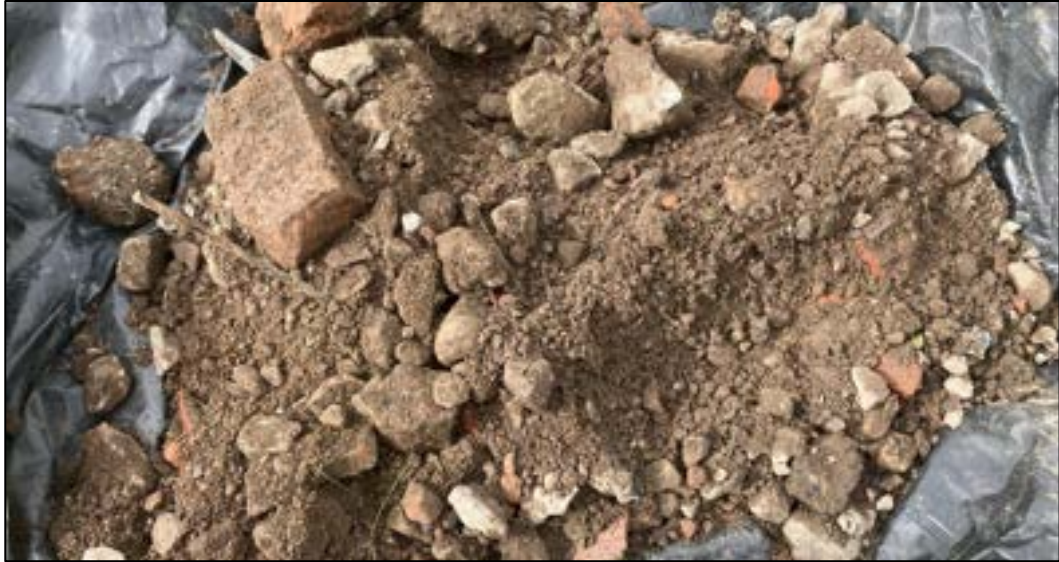
Figure 4-8: Photographic record of the soil profile at HP16A, comprising coarse grained soils
