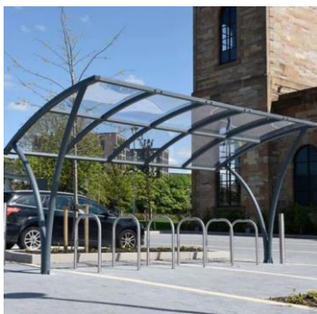
3.17 Bicycle Stands : Broxap Apollo or similar approved, colour coated (to shelter frame). Sheffield type stands fixed to concrete pads or bases below the paving floor finish. Layout to achieve minimum number of bicycle space provision indicated to comply with planning guidelines and requirements. Bike Hoops to be stainless steel.
