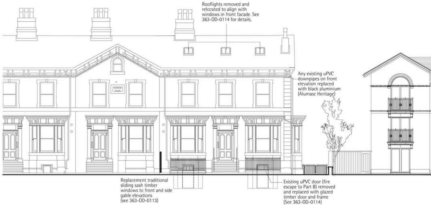
NW Elevation (As Proposed) 1:100
