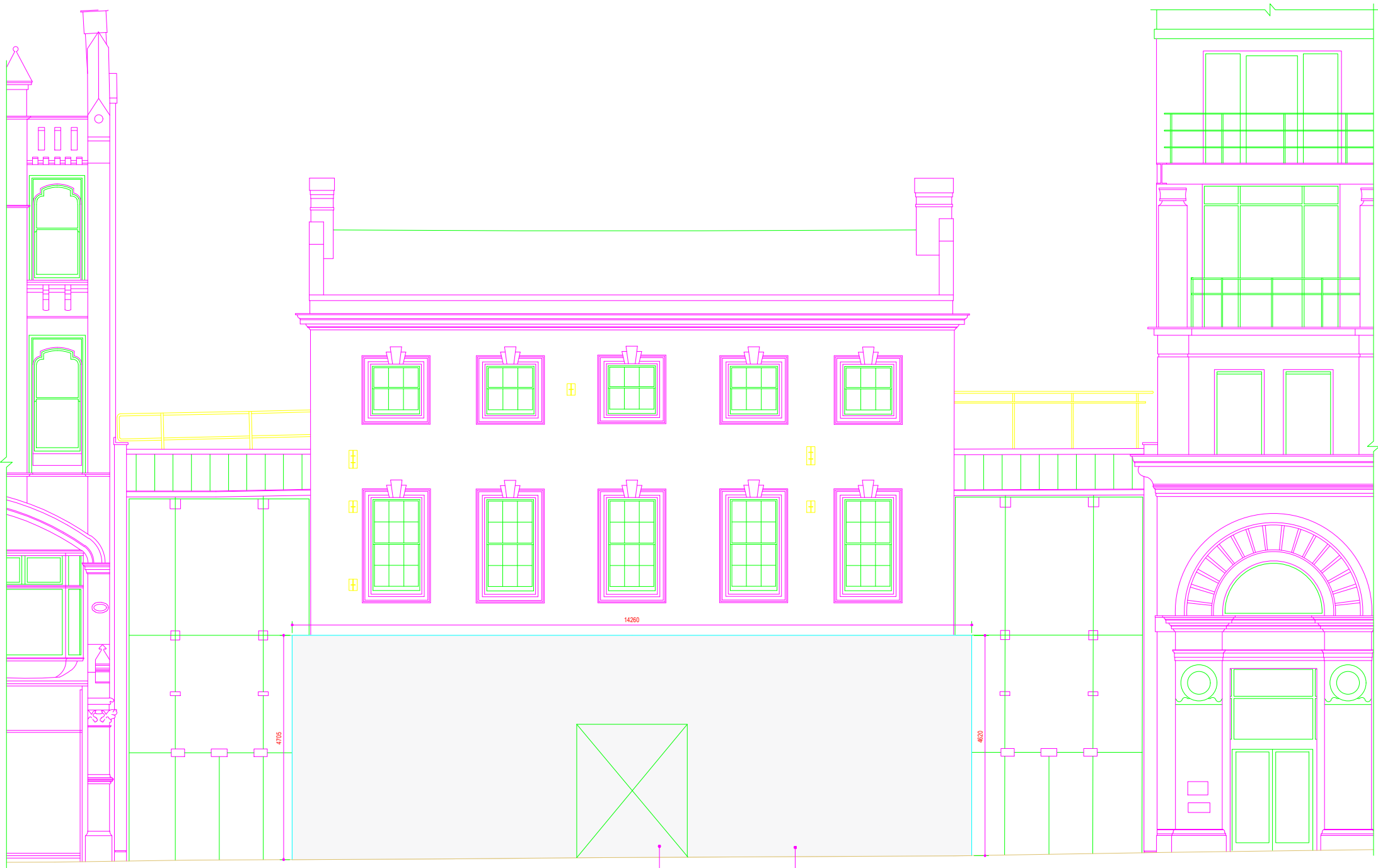
1 PROPOSED HOARDING FRONT ELEVATION - KING STREET SCALE: 1:50@A1; 1:100@A3
