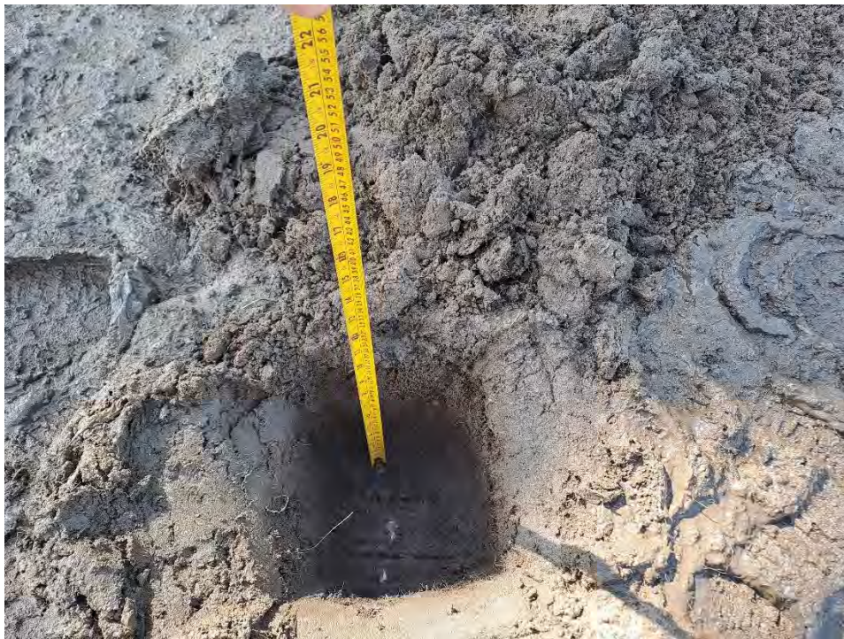
Plate 10: Sports Pitch Validation (SP09) showing approx. 270mm topsoil prior to sand layer and turf.
