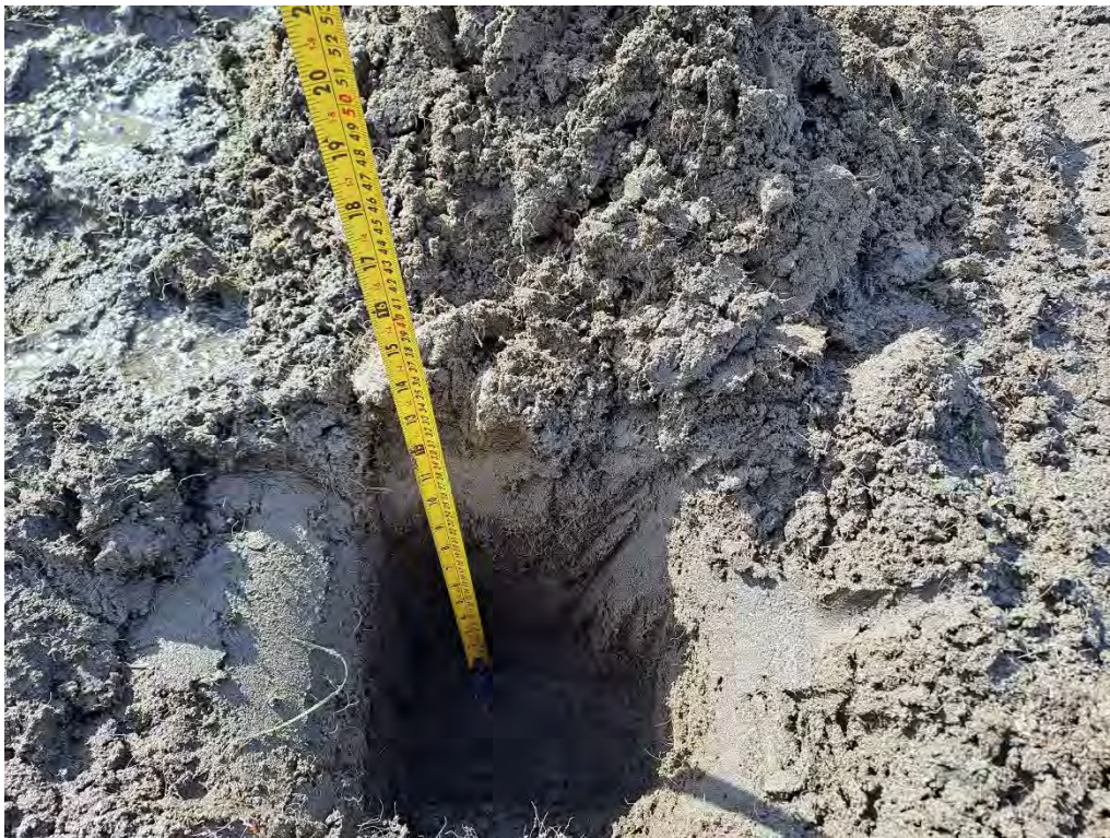
Plate 6: Sports Pitch Validation (SP05) showing approx. 280mm topsoil prior to sand layer and turf
