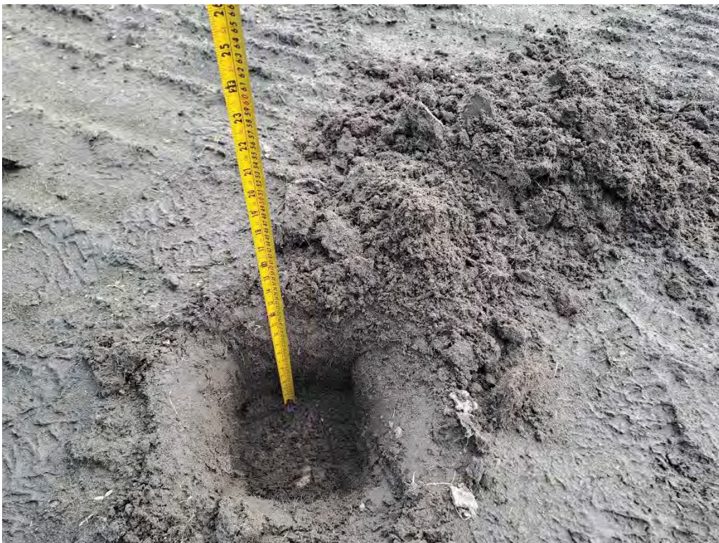
Plate 2: SP01 Validation showing approx. 270mm topsoil prior to sand layer and turf
