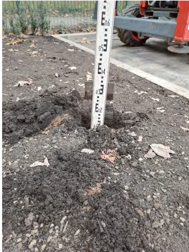
Plate 19: VP07 showing 200mm topsoil: Location Amenity Turf area adjacent to Car Park
