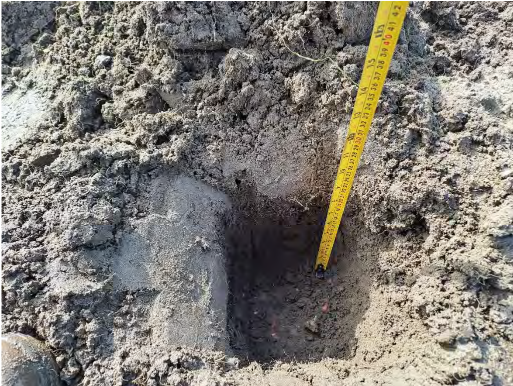
Plate 7: Sports Pitch Validation (SP06) showing approx. 270mm topsoil prior to sand layer and turf.
