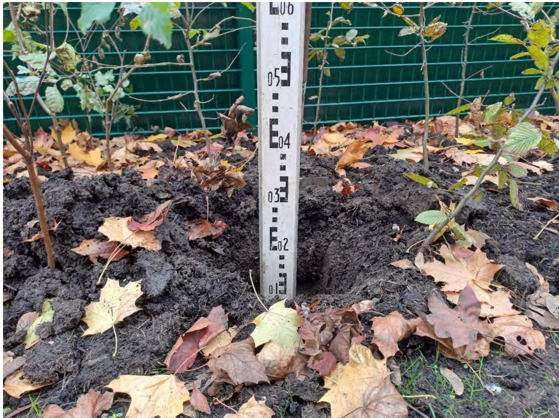
Plate 17: VP05 showing 250mm topsoil: Location adjacent to amenity turf – Habitat Area
