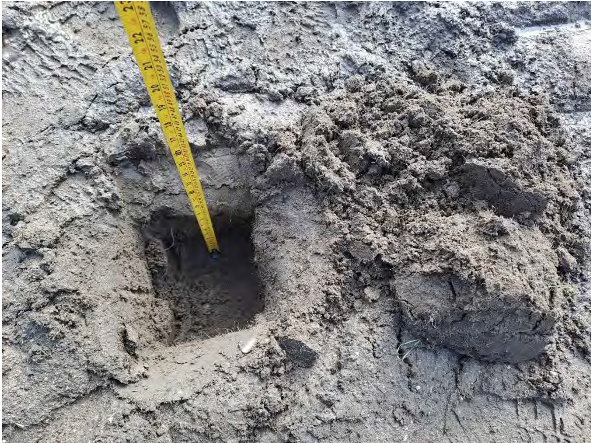
Plate 3: Sports Pitch validation (SP02) showing approx. 270mm topsoil prior to sand layer and turf
