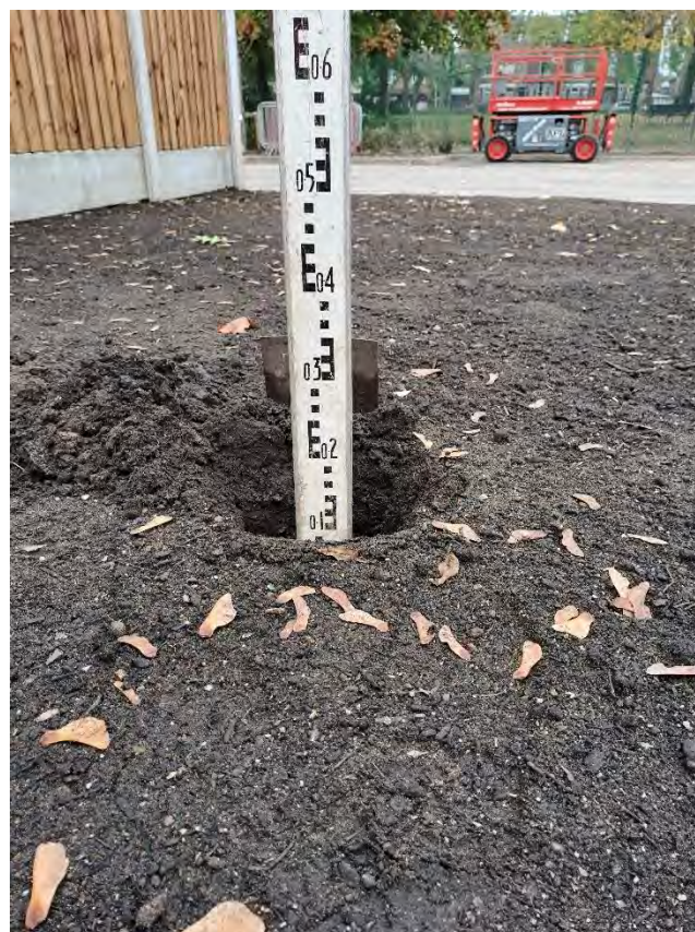
Plate 18: VP06 showing 200mm topsoil: Location Amenity Turf area adjacent to Bin Store
