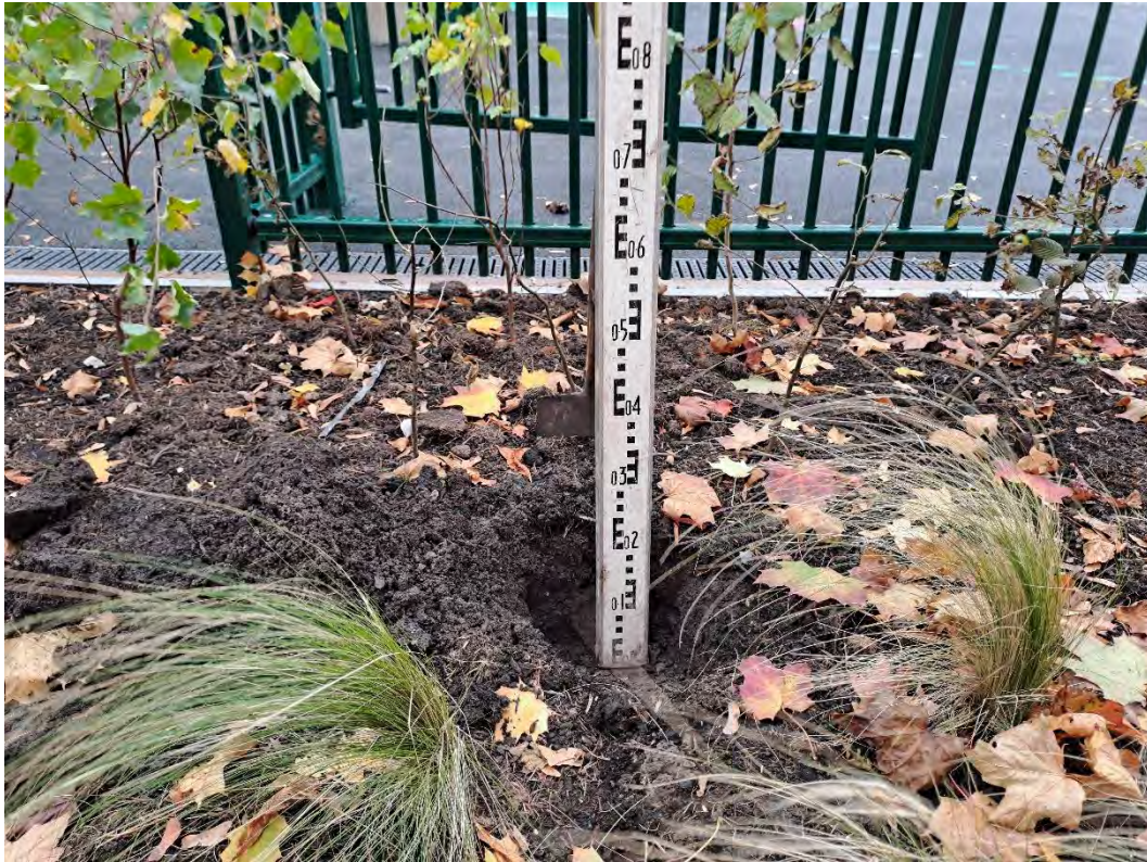
Plate 15: VP03 showing 210mm topsoil: Location Ornamental Shrub Planting - Habitat Area
