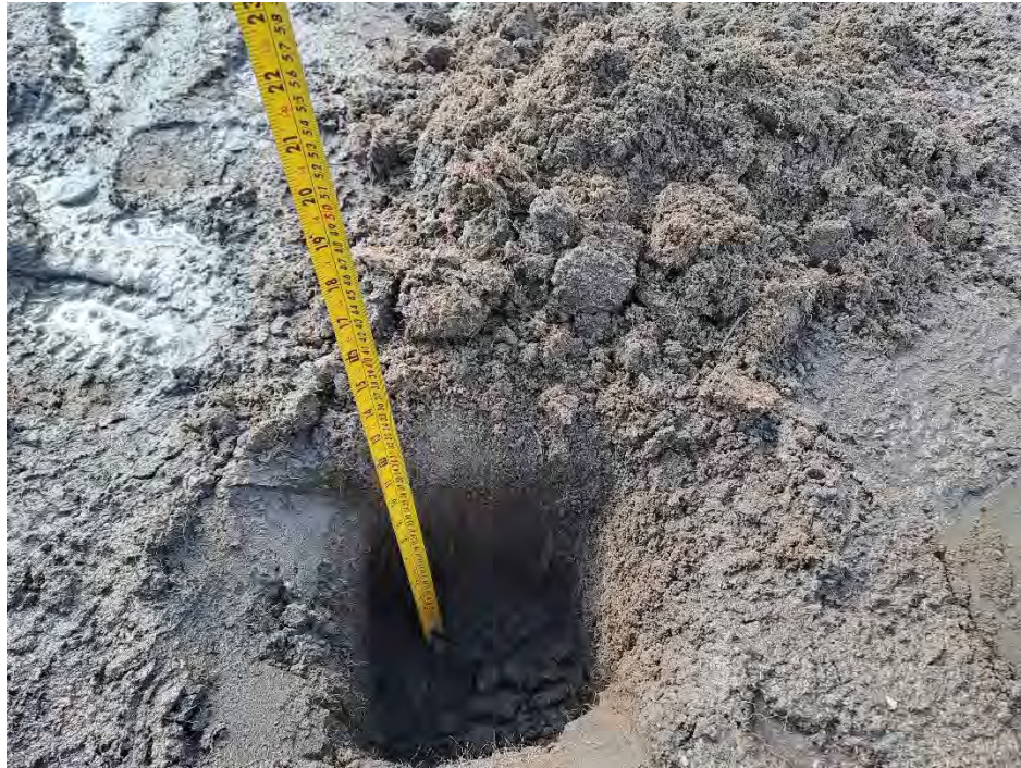
Plate 9: Sports Pitch Validation (SP08) showing approx. 270mm topsoil prior to sand layer and turf.
