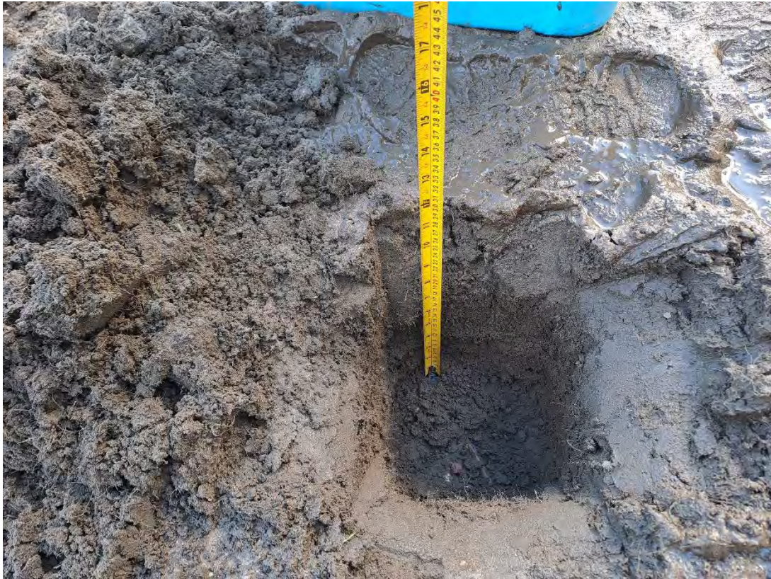
Plate 5: Sports Pitch validation (SP04) showing approx. 270mm topsoil prior to sand layer and turf
