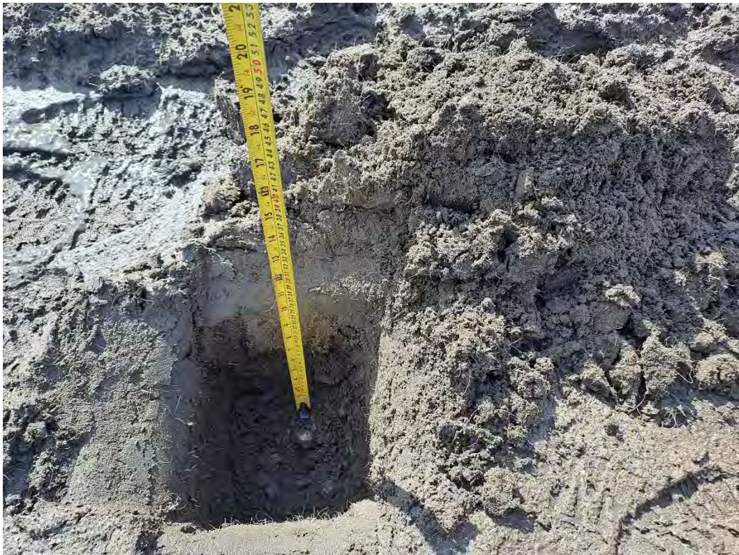
Plate 8: Sports Pitch Validation (SP07) showing approx. 270mm topsoil prior to sand layer and turf.
