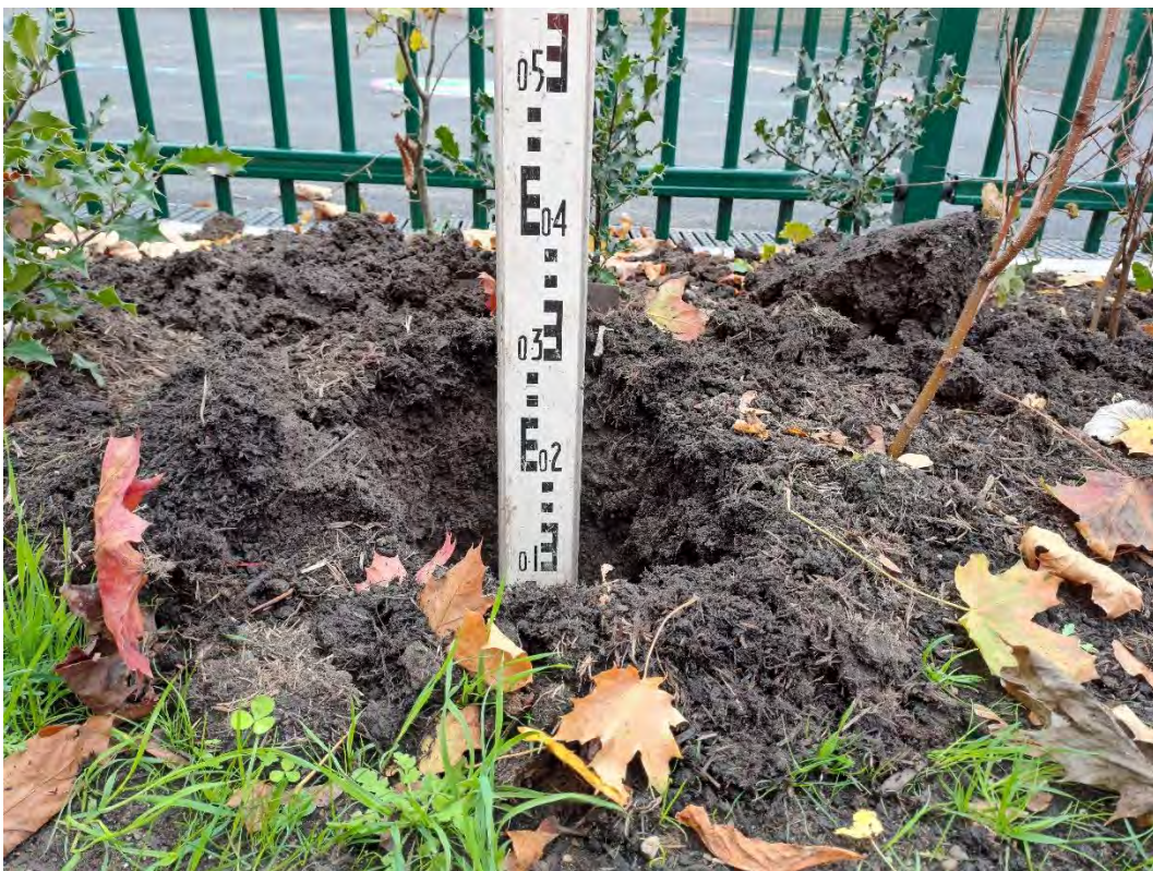
Plate 16: VP04 showing 300mm topsoil: Location Ornamental Shrub Planting - Habitat Area
