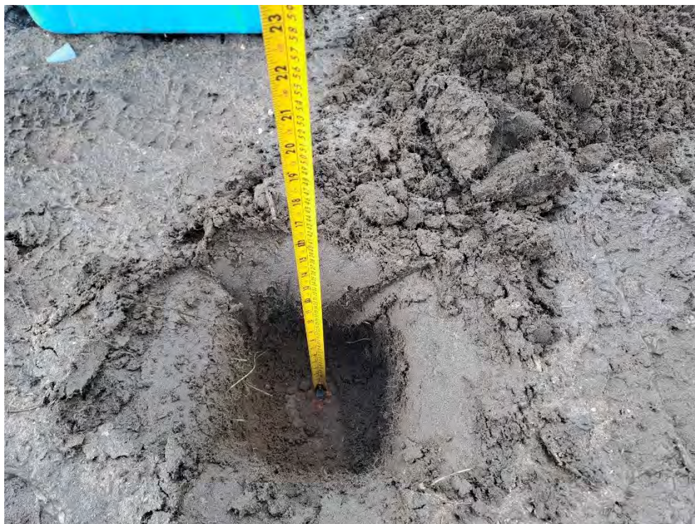
Plate 4: Sports Pitch validation (SP03) showing approx. 270mm topsoil prior to sand layer and turf
