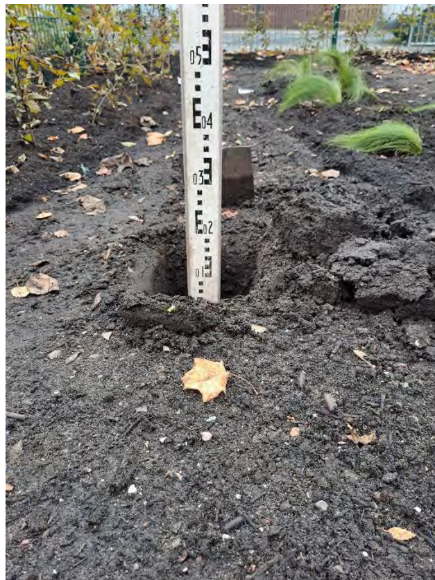
Plate 20: VP08 showing 200mm topsoil: Location Ornamental and wildflower planting Front Entrance
