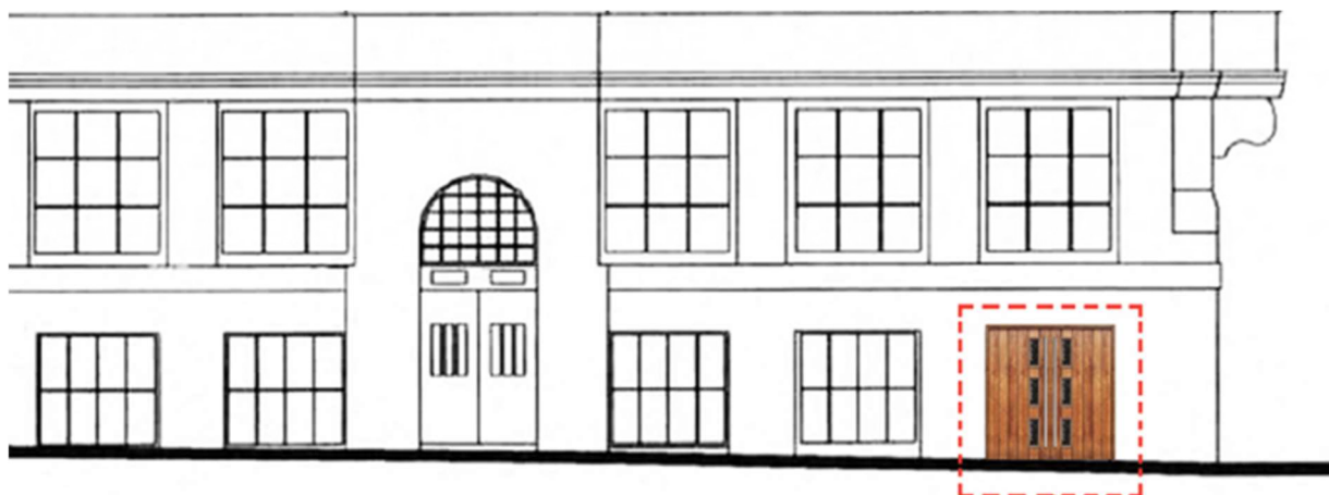
Figure 2.3 Extract from approved drawing showing doorway to be created
