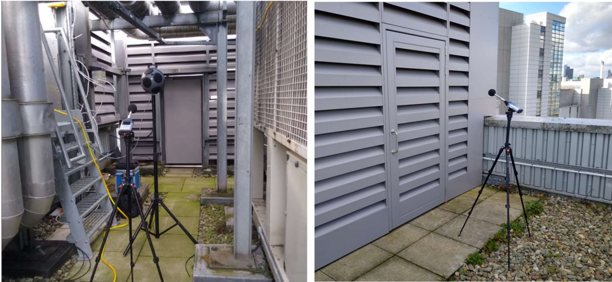
Figure 1 – Pictures of Onsite Testing Arrangement (Images Shown are Positions at 1m)
