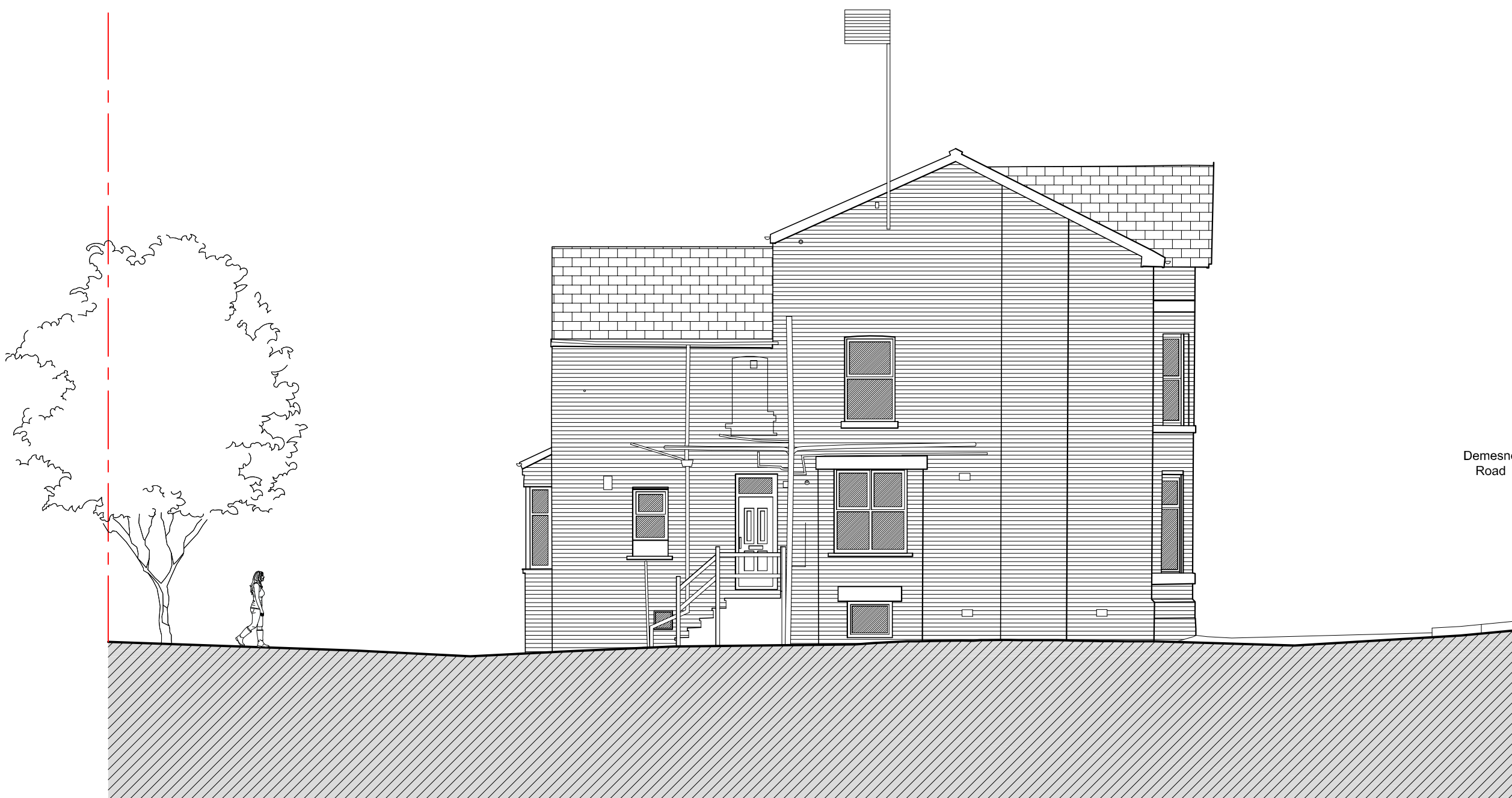
Existing West Elevation 1:100
