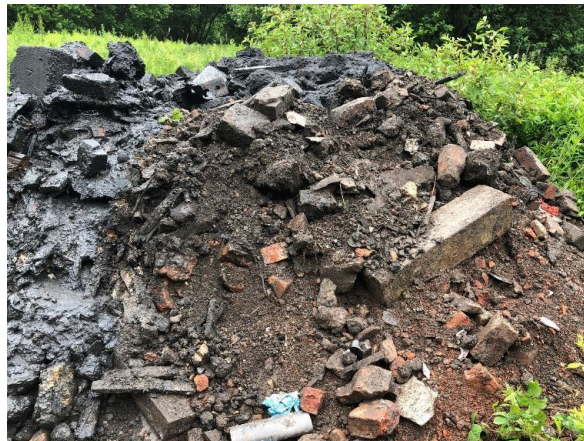
Figure 2. Example area coverage by visually hazardous materials that would be supportive of ceasing the excavation
