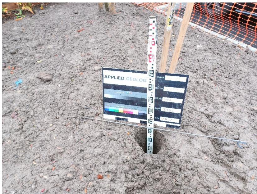
HDP4, Topsoil thickness: 450mm
