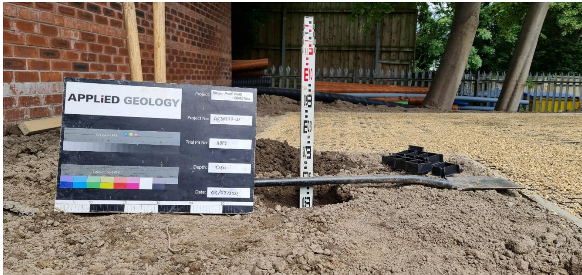
HDP1, Topsoil thickness: 600mm
