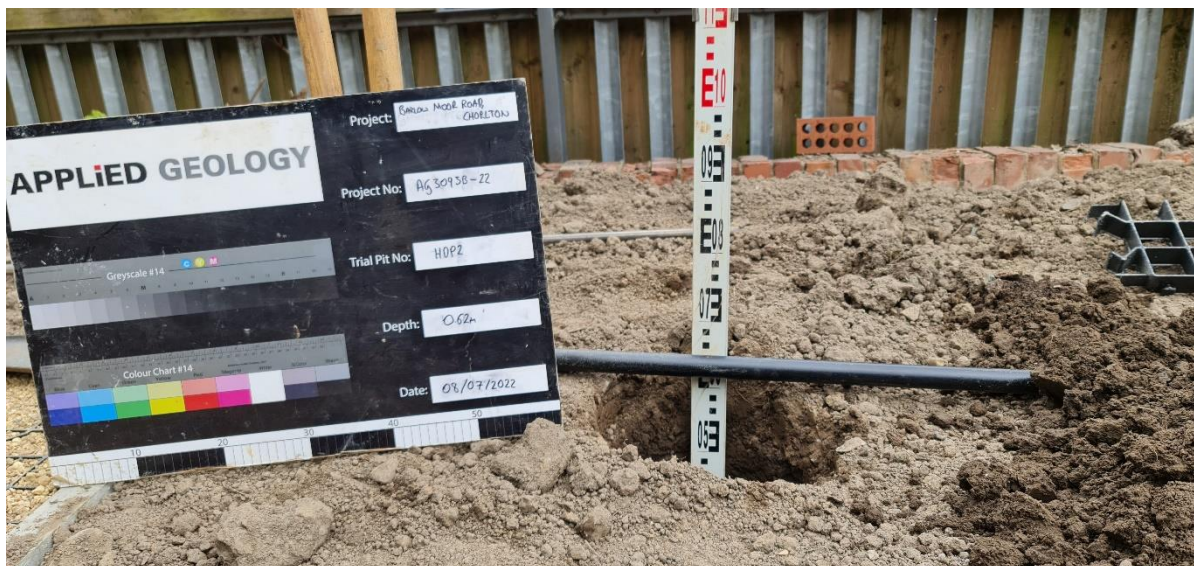
HDP2, Topsoil thickness: 620mm
