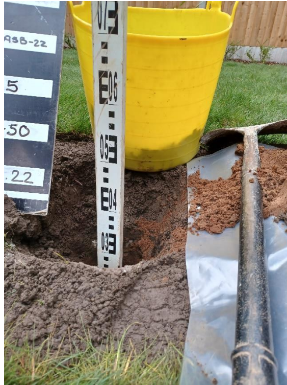
HDP5, clean cover thickness: 450mm
