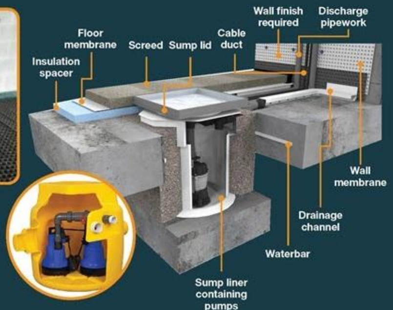
The pumping system is installed in a sump chamber, connected to the drainage channels.
