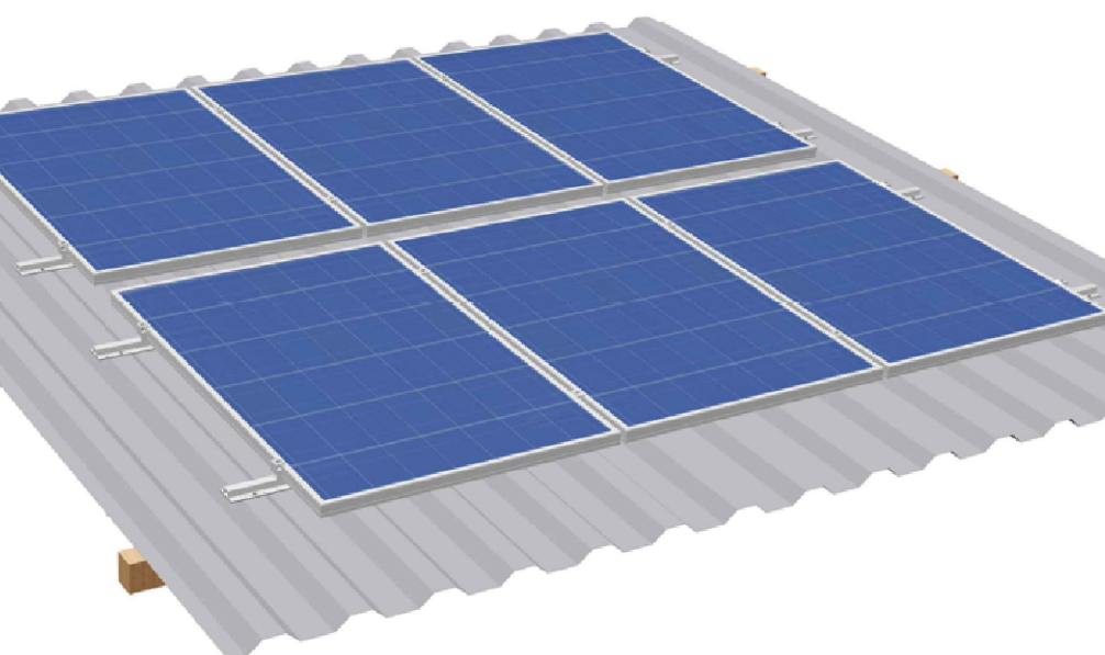
ARRAY MOUNTING VIEW
