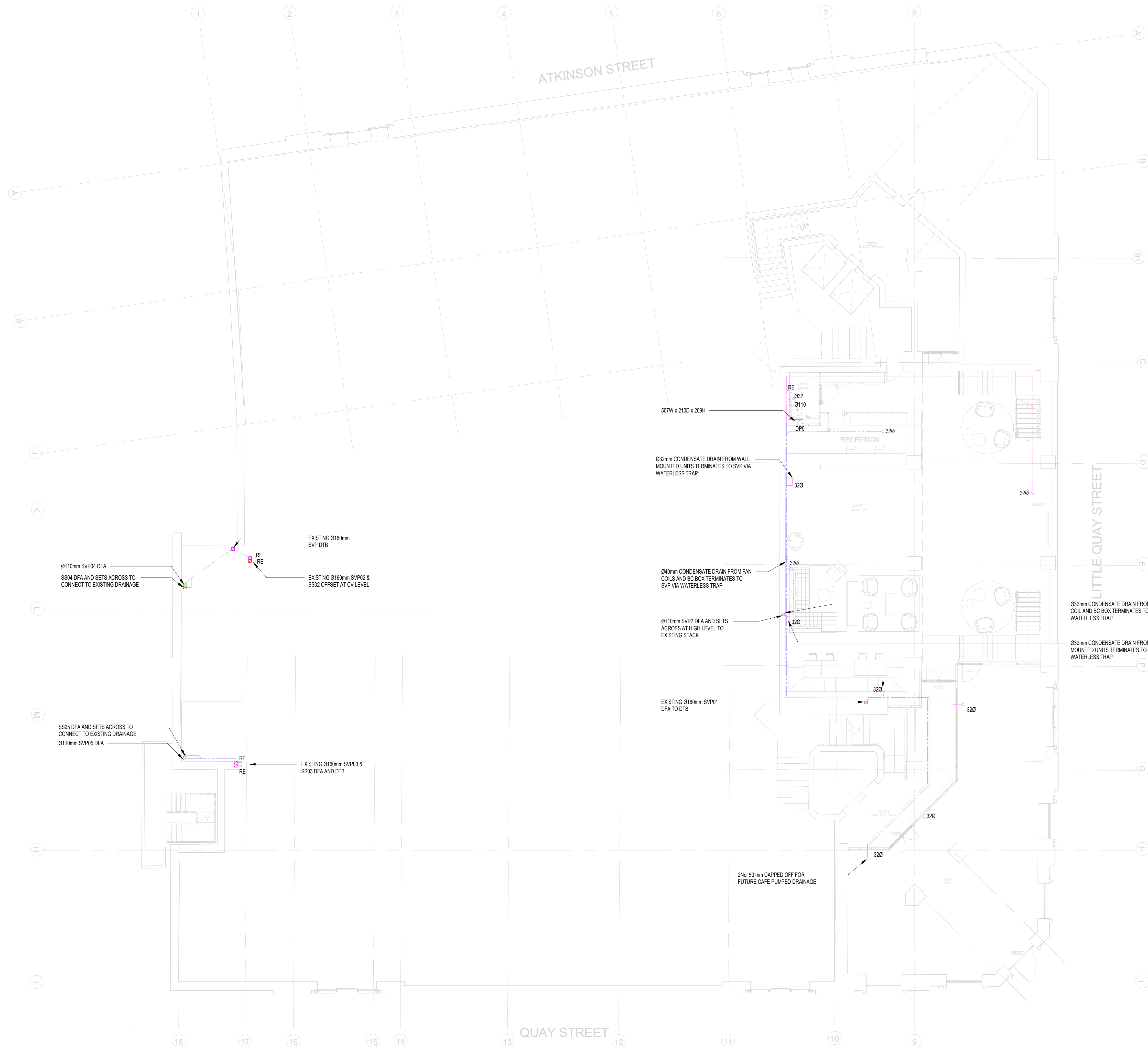
1 MECHANICAL SERVICES ABOVE GROUND DRAINAGE LAYOUT LEVEL 00 1 : 100
