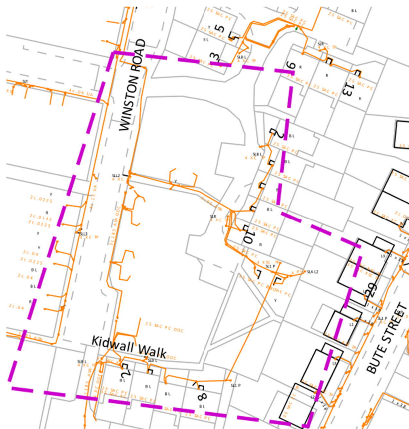
Figure 5.1 – Existing Electricity Infrastructure Plan
