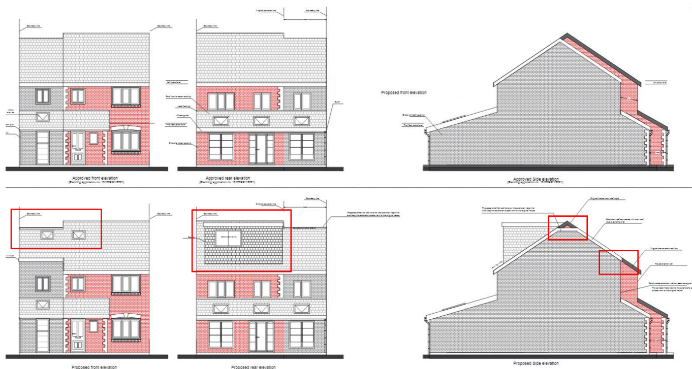
Image 1 Comparison between the approved drawings (top) and the proposed (below).
