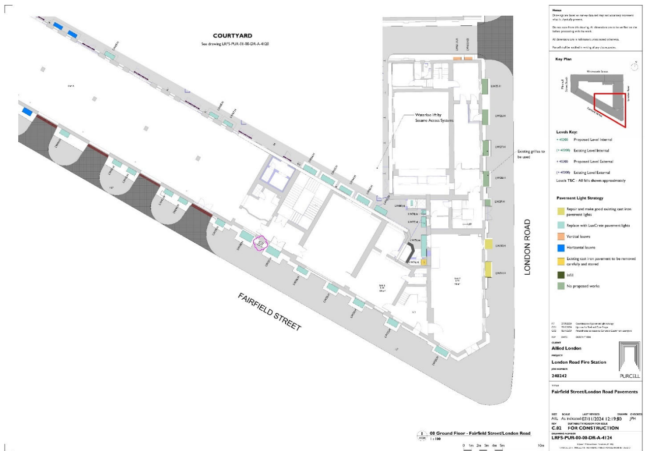
Figure 6 – Fairfield St/London Road Pavement Light Strategy
