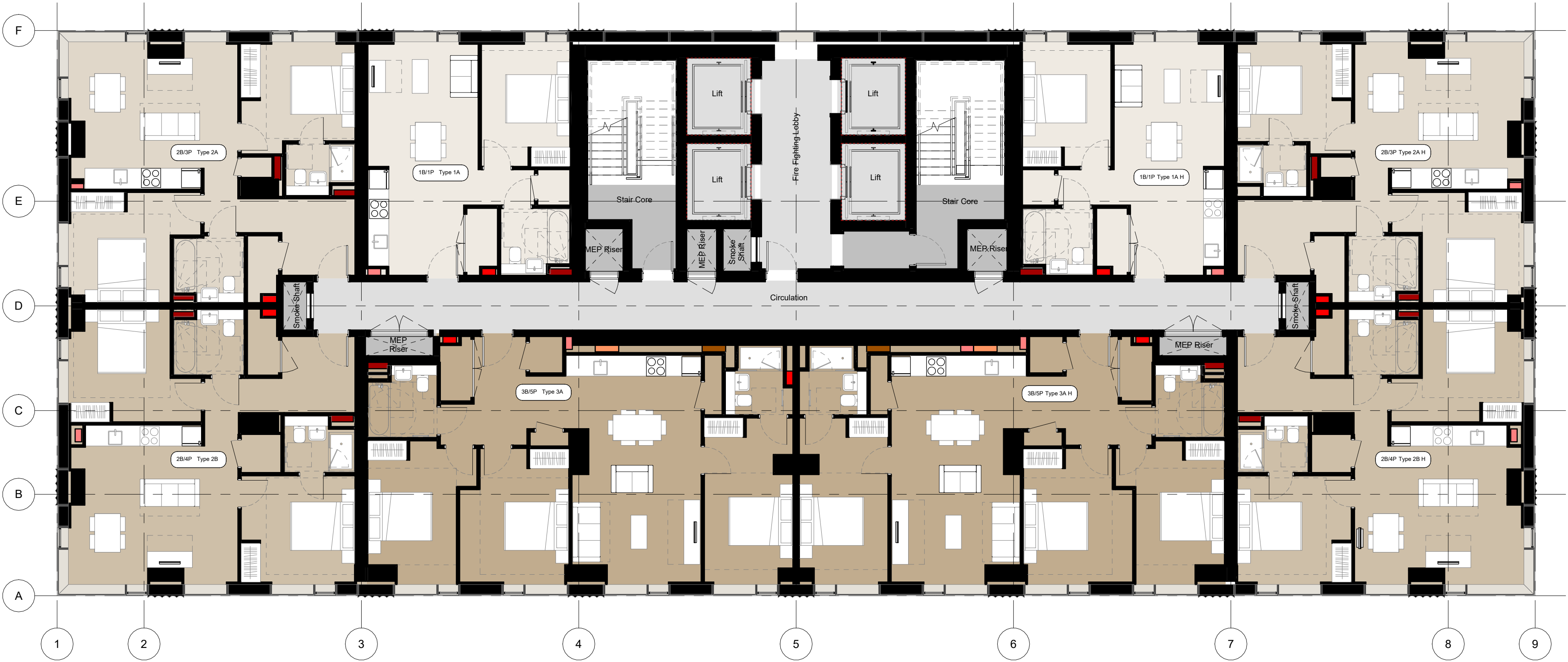
General Arrangement - Typical Floor Levels 34-40 (3 Bed Arrangement) 1 : 100
