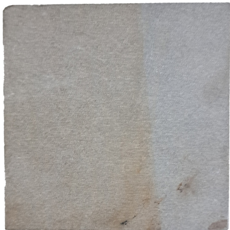
Sandstone, flamed DGH, Sandstone Natural To be used on public footpath. Sandstone sizes and pattern to match existing sand-
