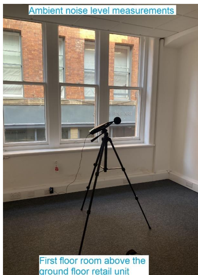
Figure 3.1. Ambient noise level measurements carried out inside the first floor room facing Ridgefield. Room windows are closed.
