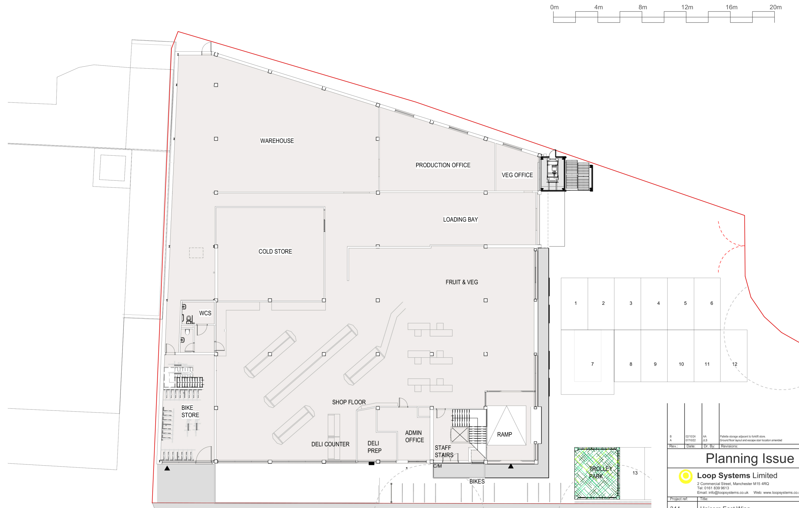
Proposed Ground Floor Plan Scale: 1:200
