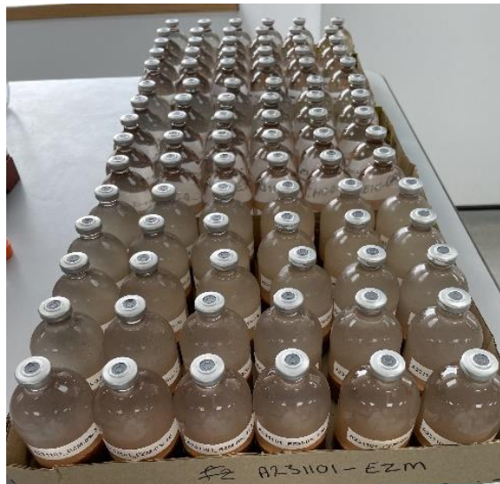
Photo: bench Scale Kinetic reactors
