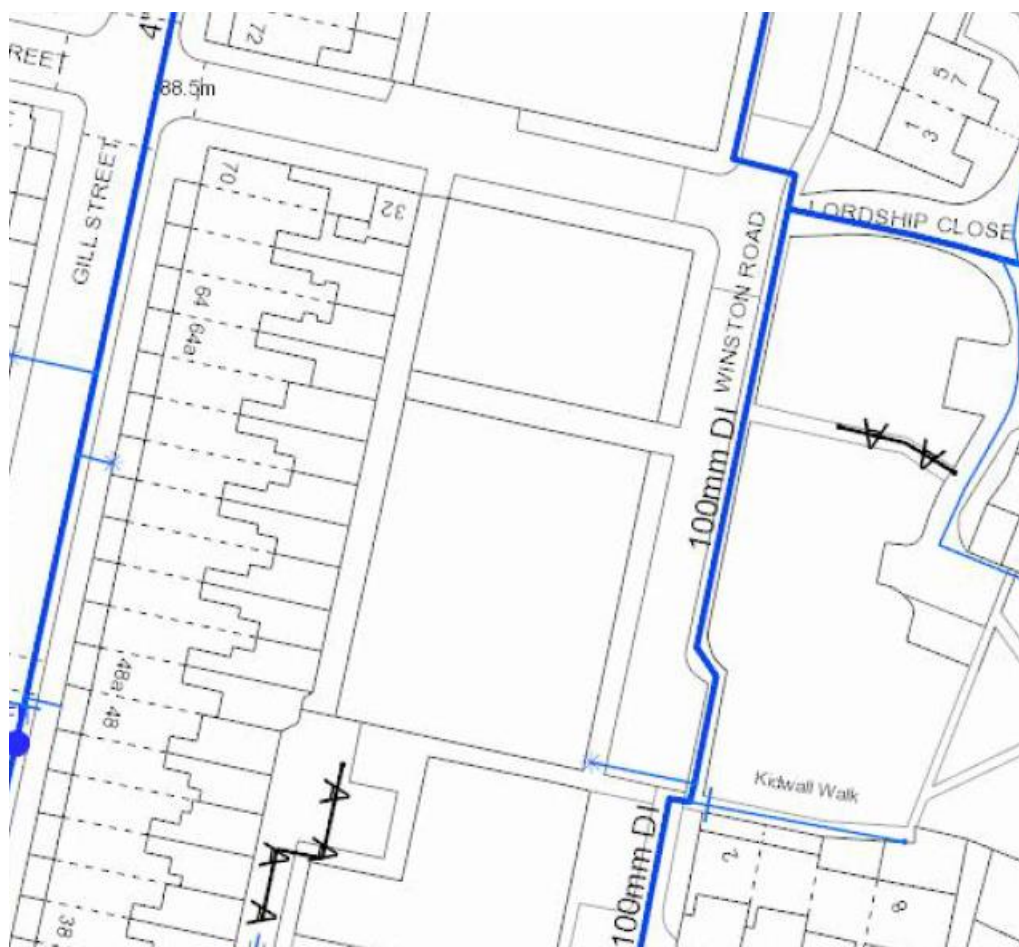
Figure 7.1 – Existing water infrastructure plan
