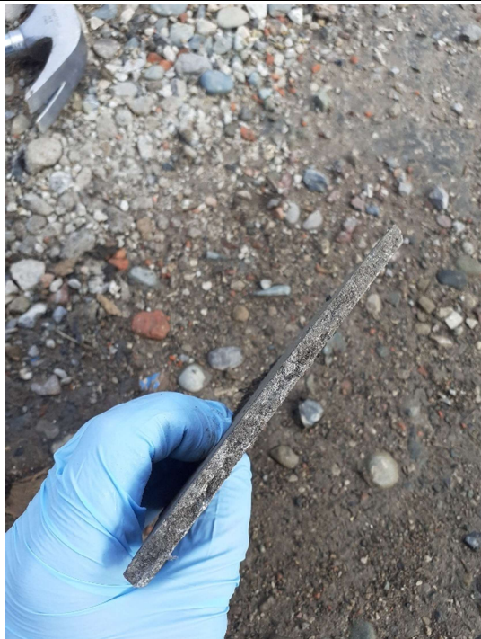
Plate 33: Monday 5 th September 2022. Asbestos cement fragment from site excavations.
