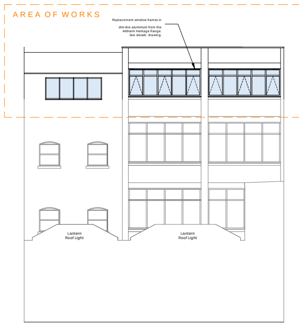
Proposed External Elevation F.
