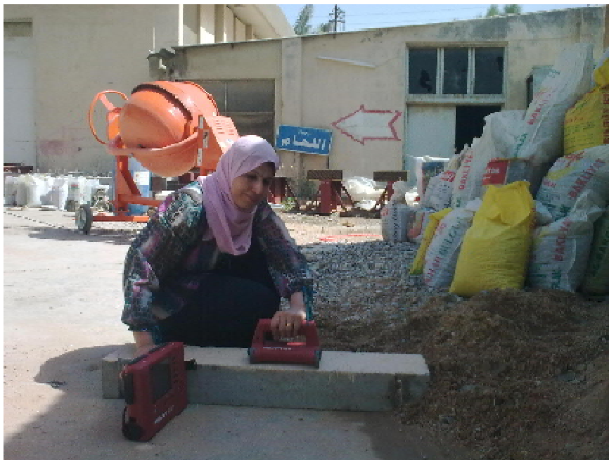
Figure (2) Testing of sample by Ferrscan
