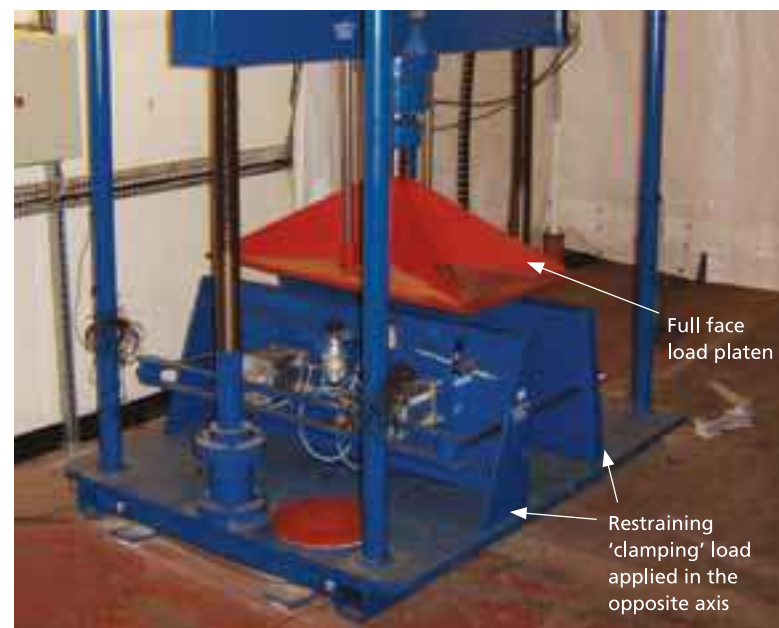
Figure 8 Compression test rig
