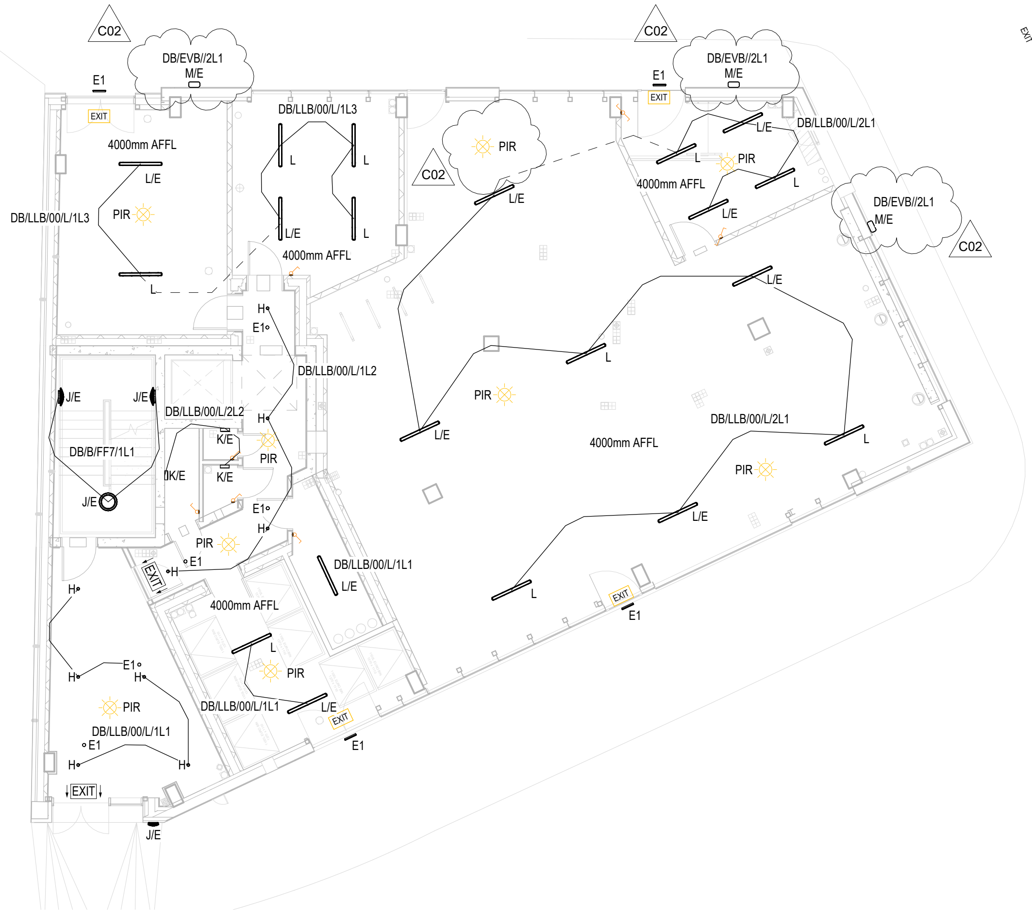
1 Block B - Level 00 - Lighting Layout 1 : 100
