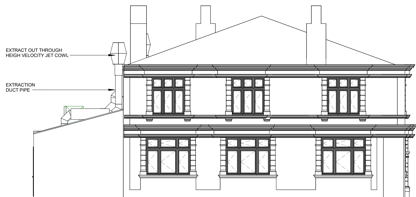
4 Existing Left side Elevation.. 1 : 100
