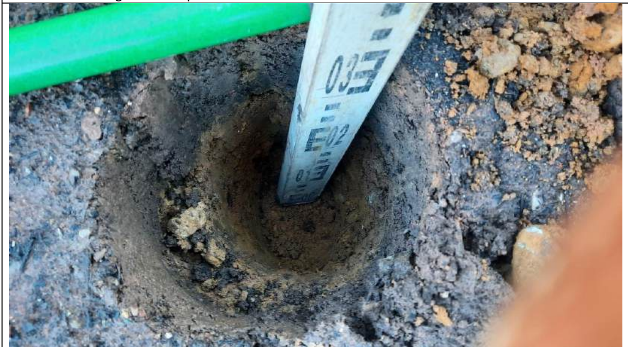
Photo 6 – Showing Plot 16 depth validation to 0.30m.
