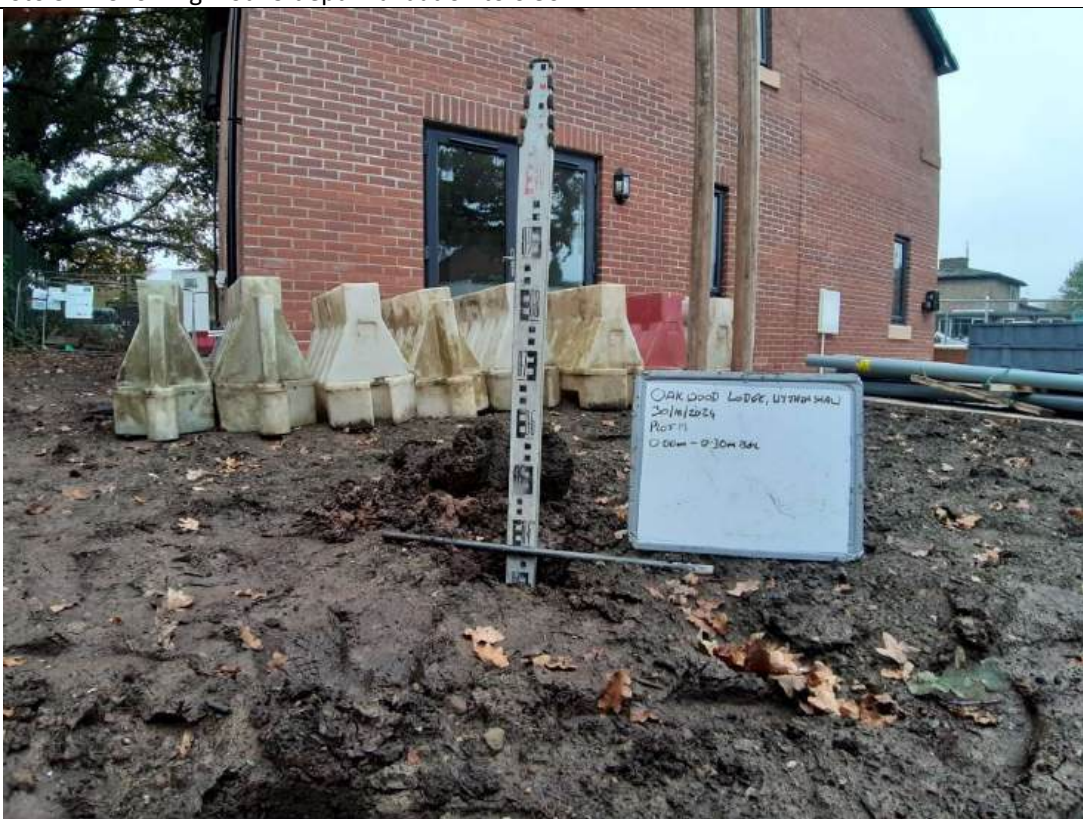
Photo 32 – Showing plot 19 depth validation to 0.30m.
