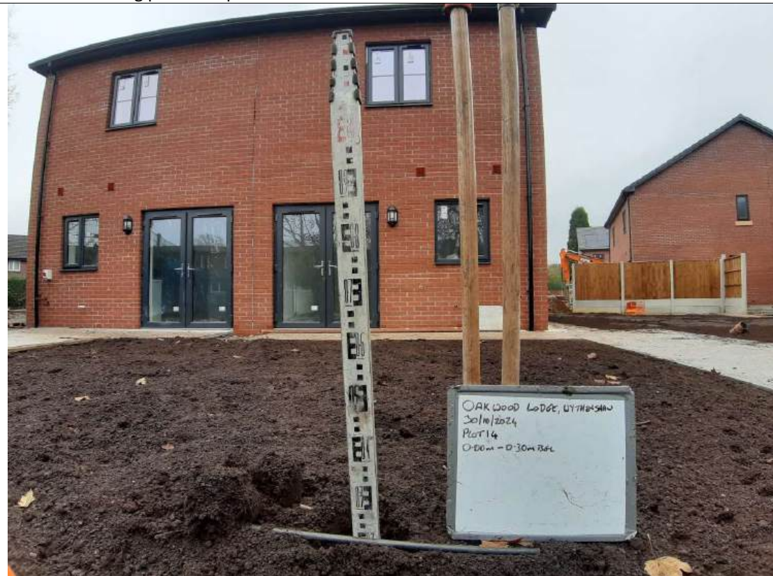
Photo 26 – Showing Plot 14 depth validation to 0.30m.
