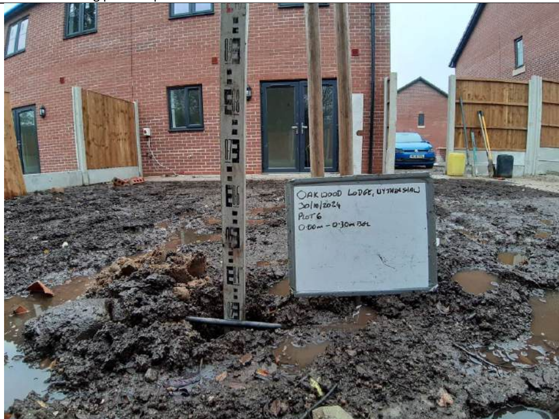
Photo 10 – Showing plot 6 depth validation to 0.30m.
