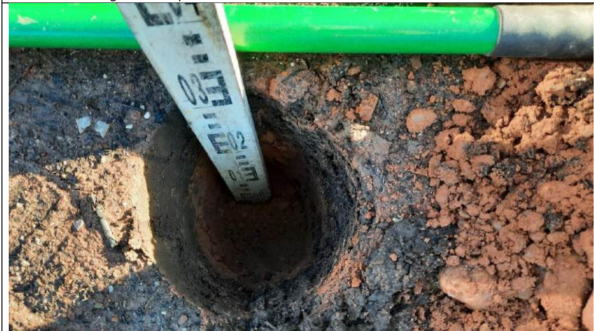
Photo 4 – Showing Plot 15 depth validation to 0.30m.
