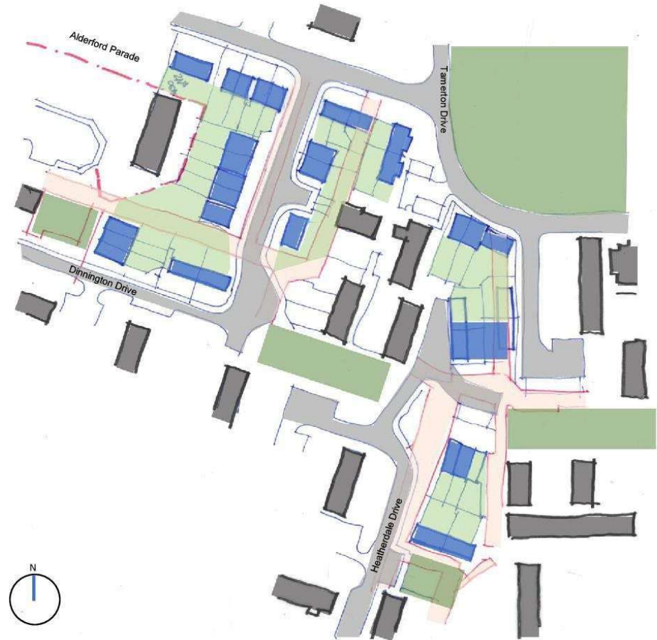
Sketch Site plan illustrating an adjusted site plan which looked to minimise the impact of the below ground services
