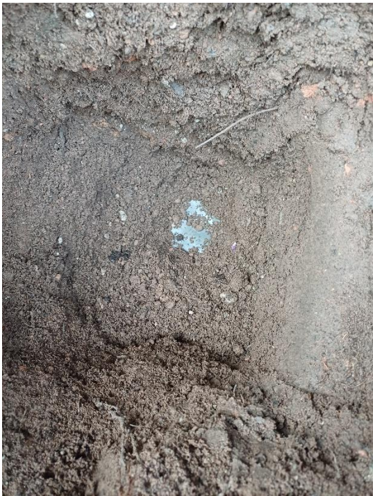
Plate 20: Look downhole at MTH106, showing membrane as the base of the hole.
