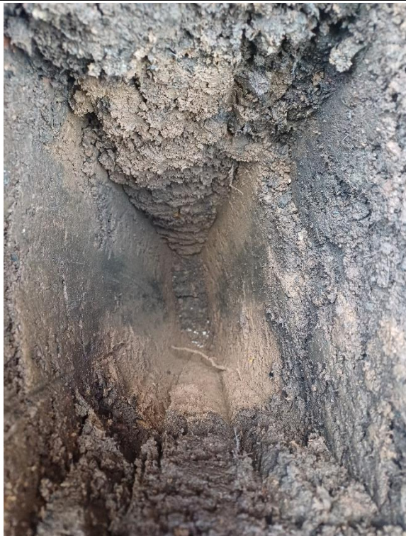
Plate 5: The bottom of MTH101. Estimated topsoil: 400mm, estimated subsoil: 430mm.
