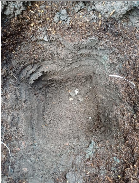
Plate 30: Look downhole at the tree pit at MTH110, showing concrete as the base of the hole.
