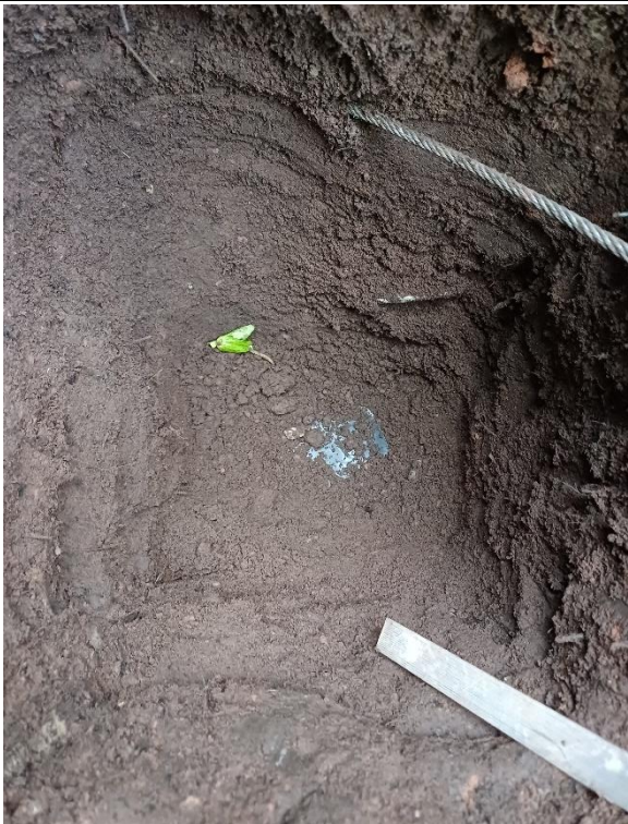
Plate 27: Look downhole at MTH109, showing membrane as the base of the hole.
