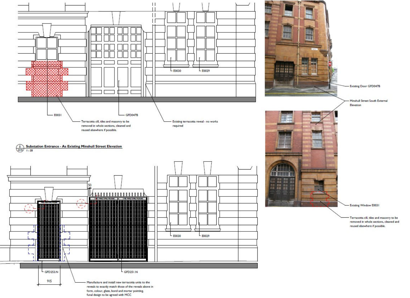
Figure 2 – Substation Gates Elevation Existing and Proposed
