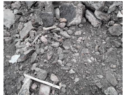
Item 15 - Spoil stack adjacent trial pit 13 - Bitumen pipe debris on and mixed in the spoil stack
