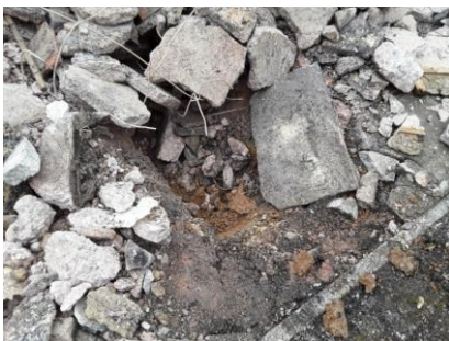
Item 7 - Trial pit 7 - Soil sample taken from the top 200mm layer, beneath the concrete
