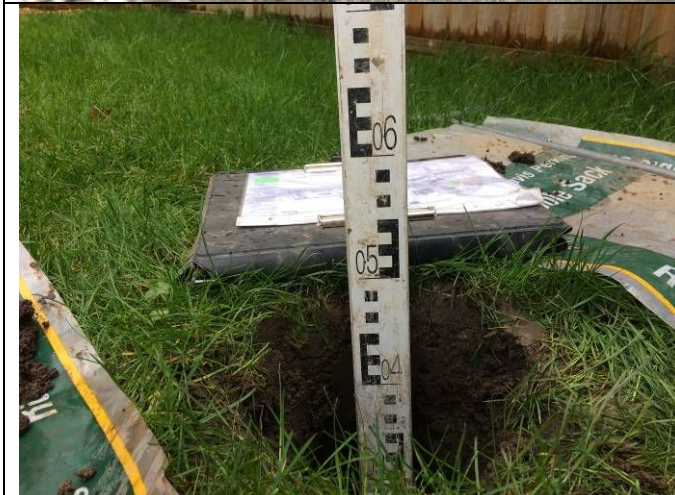
Photograph 12: Depth measurement in rear garden of Plot 41.
