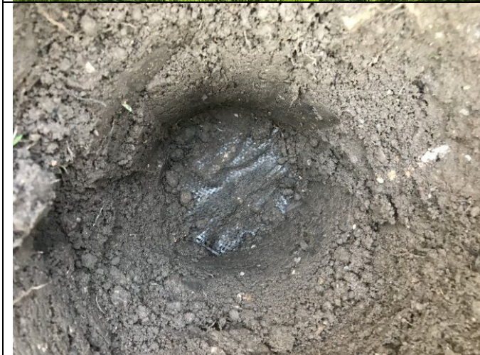
Photograph 14: View of soil in capping layer excavation in rear garden of Plot 37 with geotextile membrane visible.
