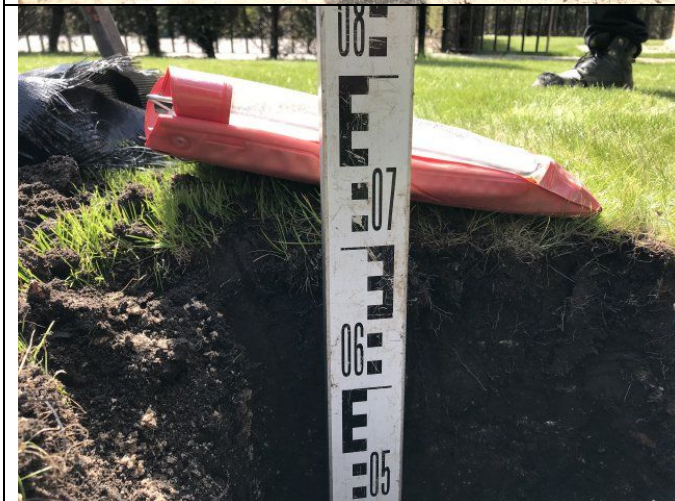
Photograph 31: Depth measurement in rear garden of The Lodge.
