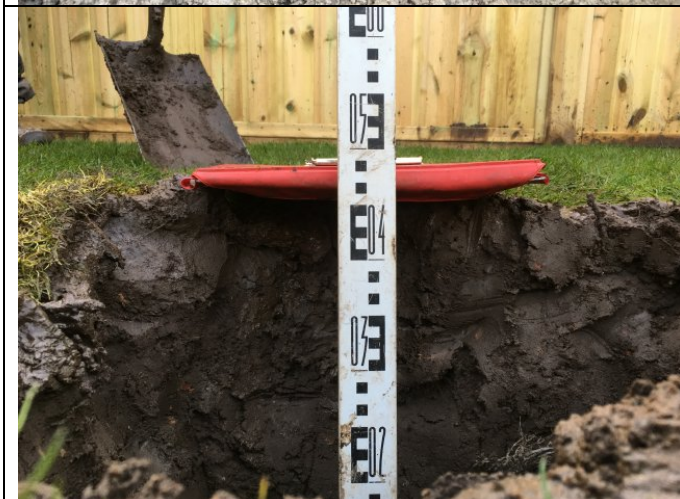
Photograph 6: Depth measurement in rear garden of Plot 31.
