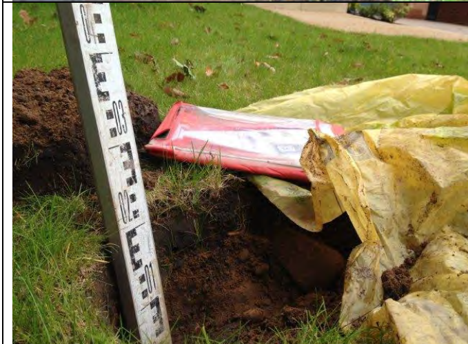
Photograph 12: Depth measurement in front garden of Plot 11.
