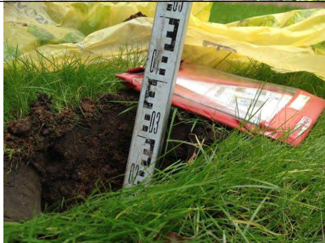
Photograph 48: Depth measurement in front garden of Plot 17.
