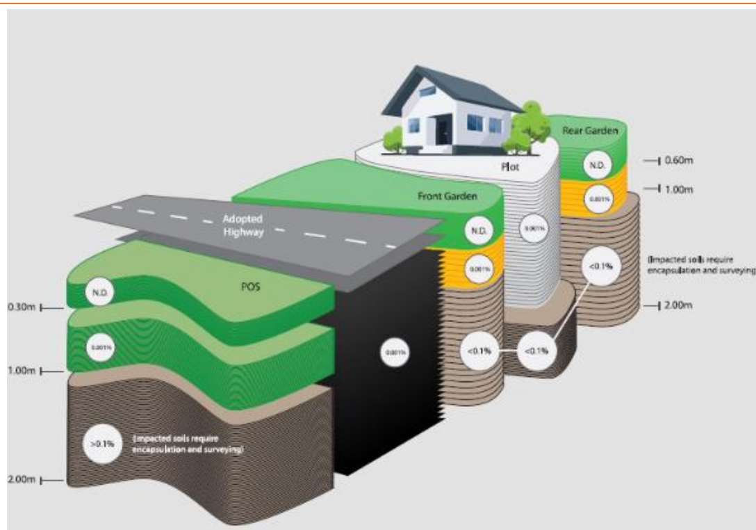
FIGURE 4.1 ASBESTOS RISK MITIGATION CONCEPTUAL SITE MODEL
