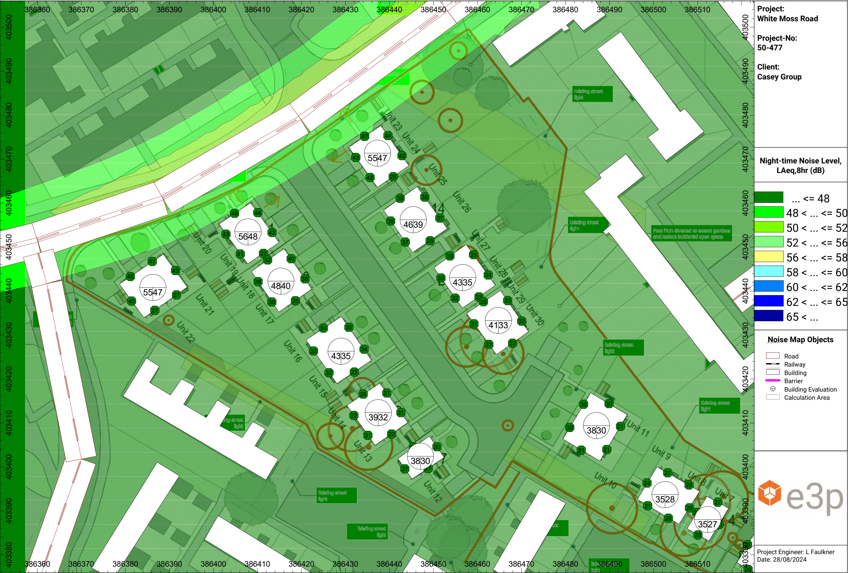
Figure 4 - Night-time Grid Noise Map - Grid calculated at a height of 4 m above ground level
