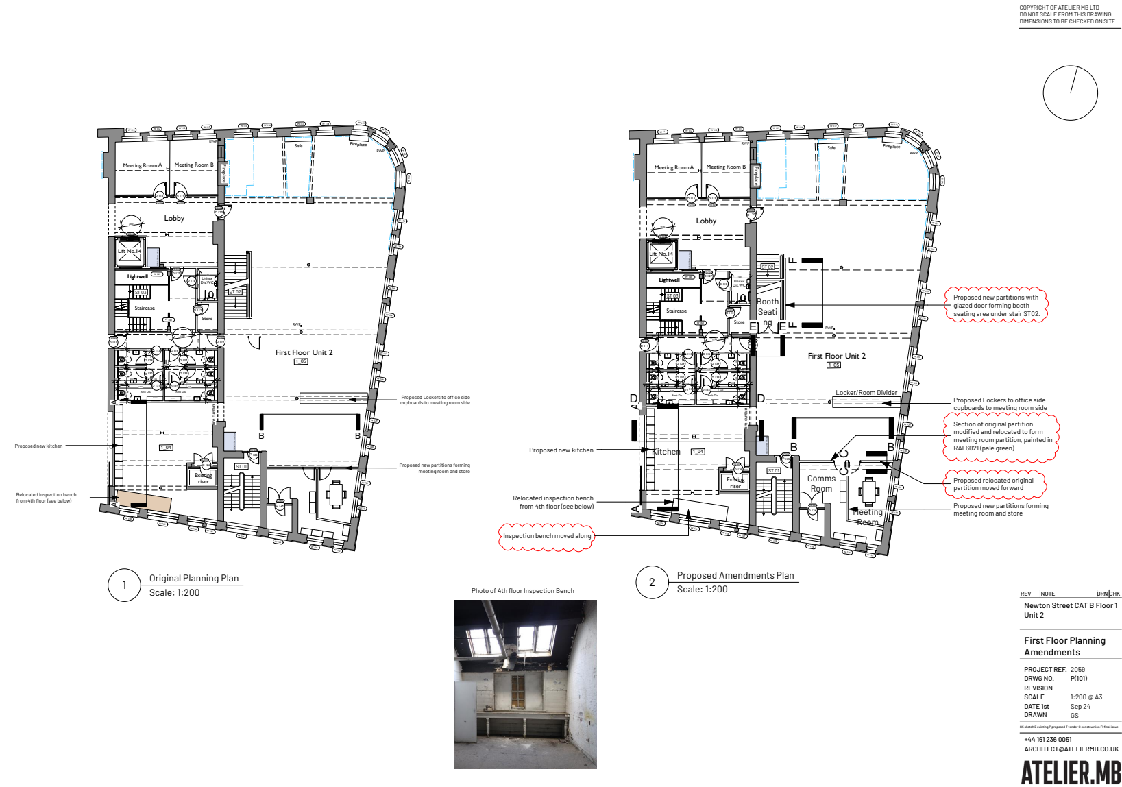
Image: Previous proposals alongside amended proposals and image of inspection bench to be relocated from 4th floor.
