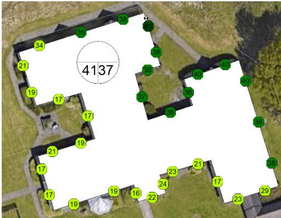
Daytime predicted noise levels at 1.5m above ground, dB L_{Aeq, 1hour}
